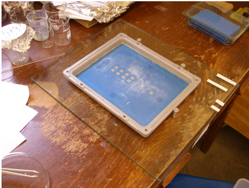
(b) Screen printing station with the 110 TPI screen. Aluminum posts adhered to the glass station base allow consistent positioning of the screen.
