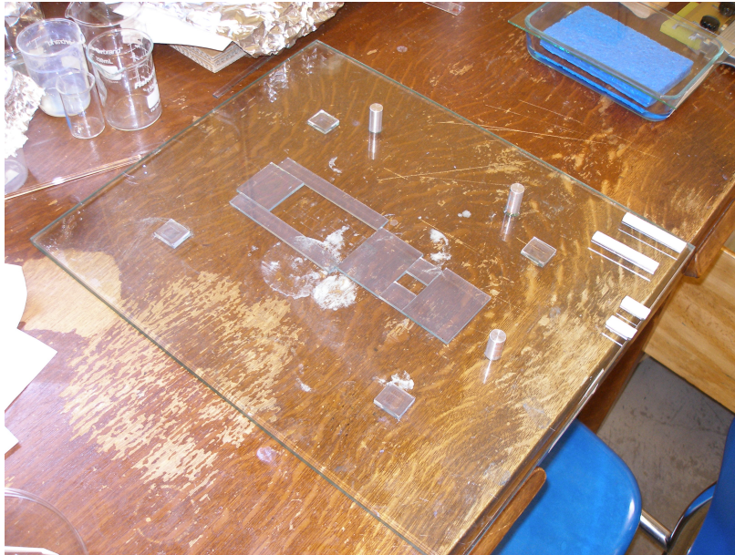
(a) Screen printing station without the screen. Pieces of FTO glass the same thickness as the substrate to be printed upon are used to keep substrates in the same position when multiple layers are printed.
