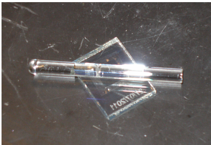
Figure 2.5: Smoothing gasket onto the substrate with stir rod. Smoothing gasket helps achieve rapid sealing without gaps in the seal.
