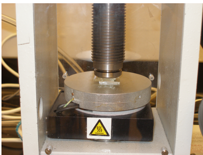
(b) Press with bottom heated platen but not the top heated platen. Cell to be sealed and extra 2.2 mm-thick glass for insulating the top platen from the cell in place.
