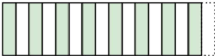
Figure 3.1: Non Unit Strided Memory Access, with stride of two
