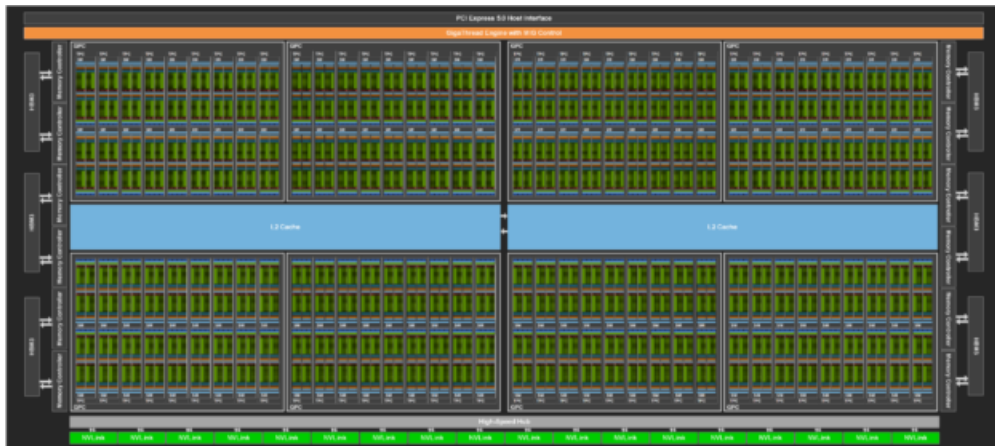
Figure 2.7: The architecture of the H100
