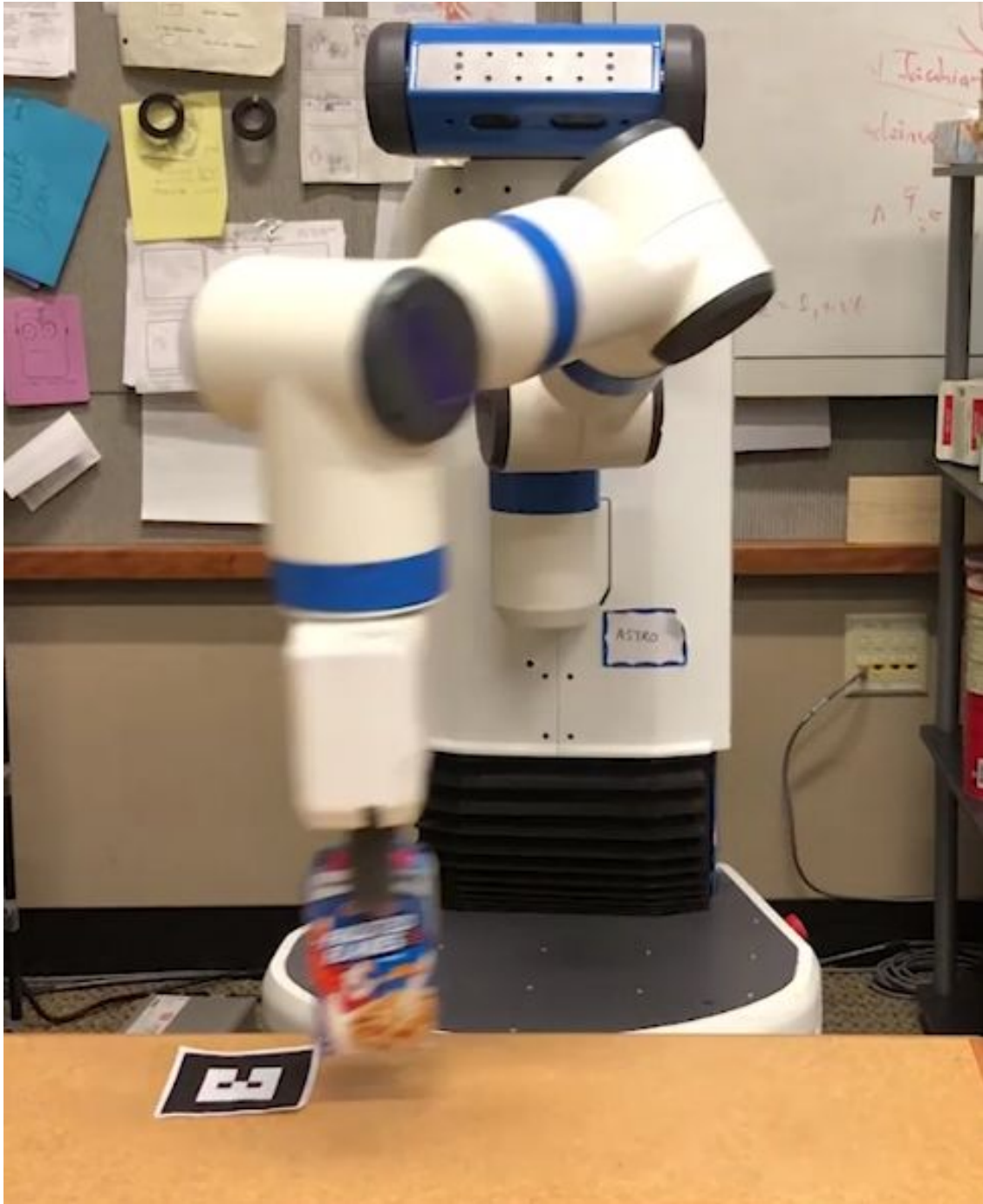
Figure 11.2: The CustomLandmarks2D prototype running on the Fetch robot.
