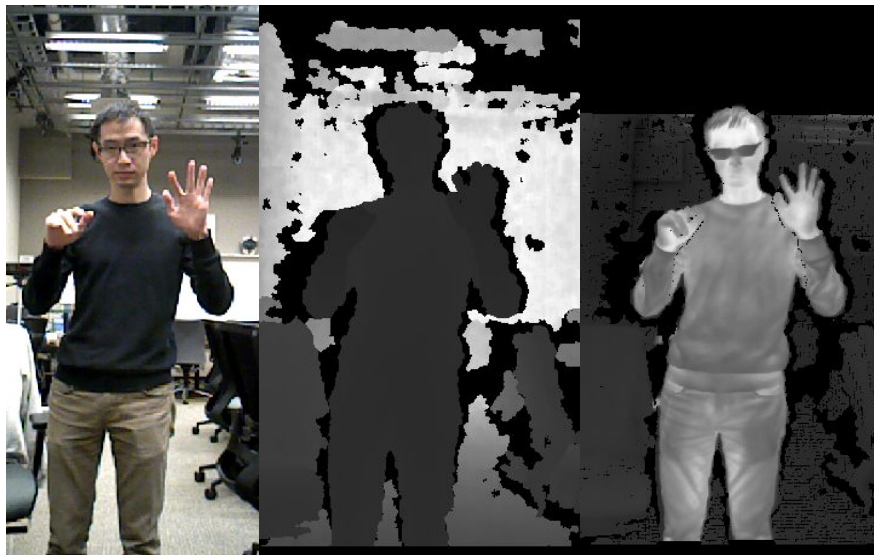
Figure 10.1: A sample set of raw images for our hand segmentation dataset. The left image is the color image, the center image is the depth image, and the right image is the thermal camera image.
