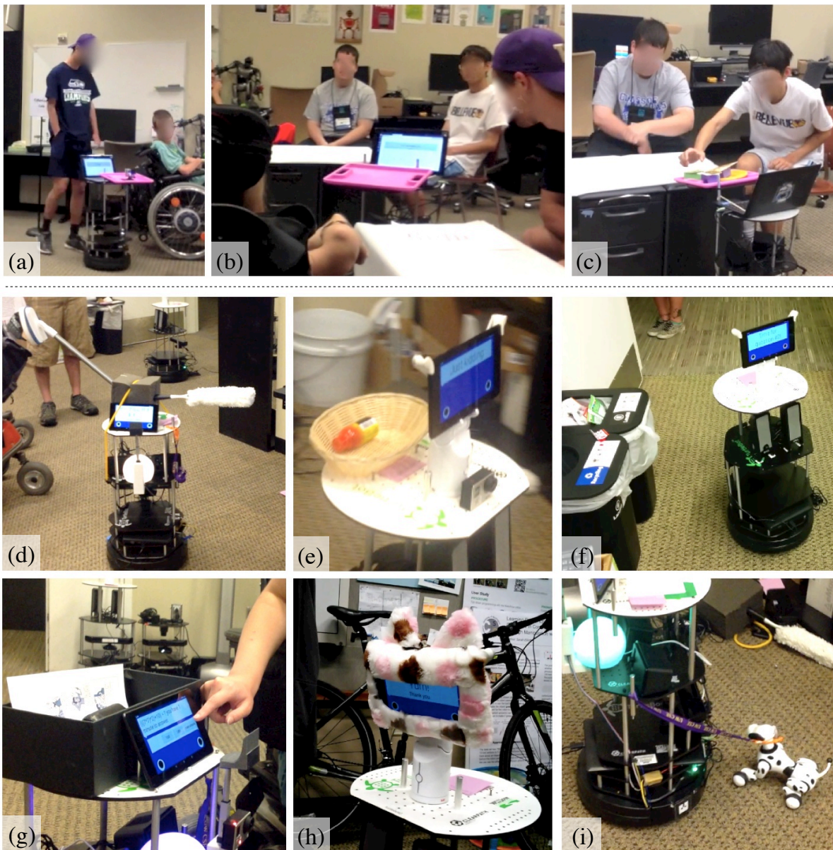
Figure 7.4: Chester, a waiter robot programmed by students at the 2015 Robot Programming Workshop, (a) escorts guests, (b) takes orders, and (c) delivers orders at “Cyber Cafe”. Robots programmed by individual students at the 2016 workshop include (d) a cleaning robot (FRED), (e) a medication reminder/delivery robot (Ultravax), (f) a language tutor robot that names objects in the room (Lærer), (g) a math tutor robot (Khan), (h) a pet robot that talks about sports (Sport), and (i) a dog walking robot (Walker).
