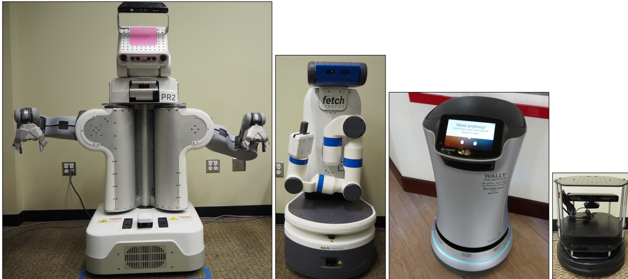
Figure 1.1: Robot platforms used in our research. From left to right, the Willow Garage PR2, the Fetch Robotics Fetch, the Savioke Relay, and the Turtlebot 2.
