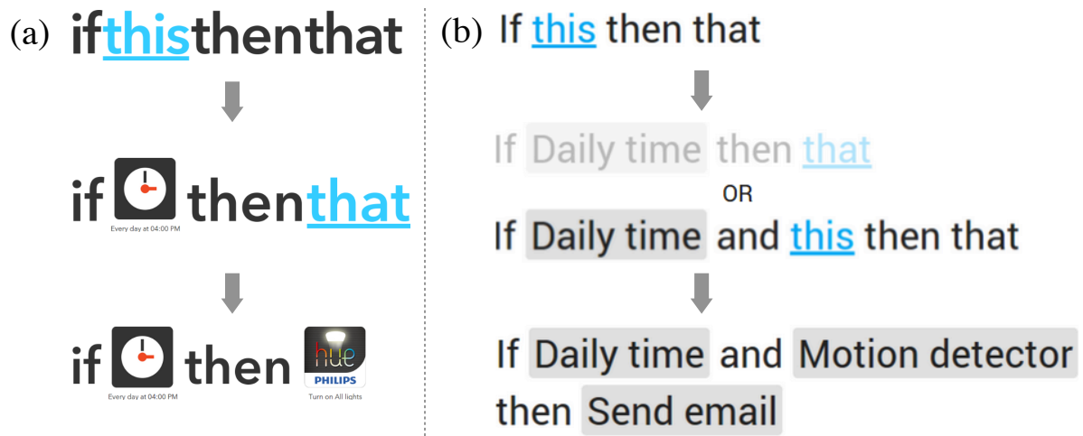
Figure 8.9: A composite screenshot of the rule creation flow in (a) IFTTT and (b) our interface.
