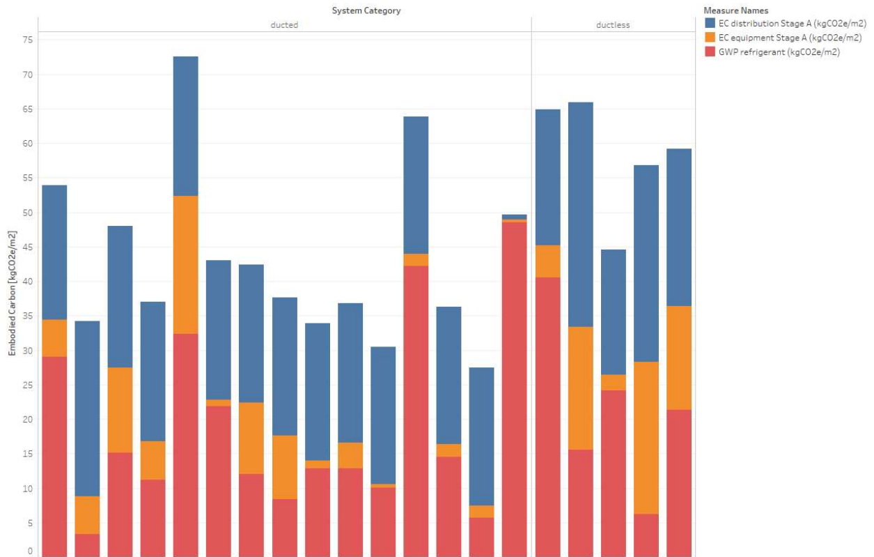
Figure 5.10 Total EC (kgCO 2 e/m 2 ) of HVAC+R systems in ducted and ductless systems HPB
