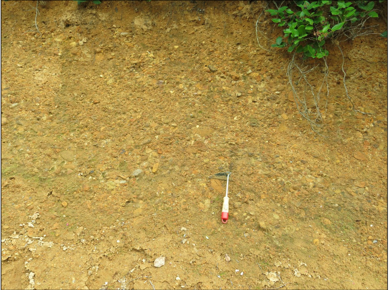
Figure A1-10. Coarse sand to gravel, with cross bedding less than 0.75 m high, dipping to west at station 20GW0922.9. Highly indurated and oxidized, with many clasts weathered through. Where identifiable, a portion of clasts are granitic and metamorphic. Unit Qgs. Scraper approximately 25 cm long. View to the southwest.
