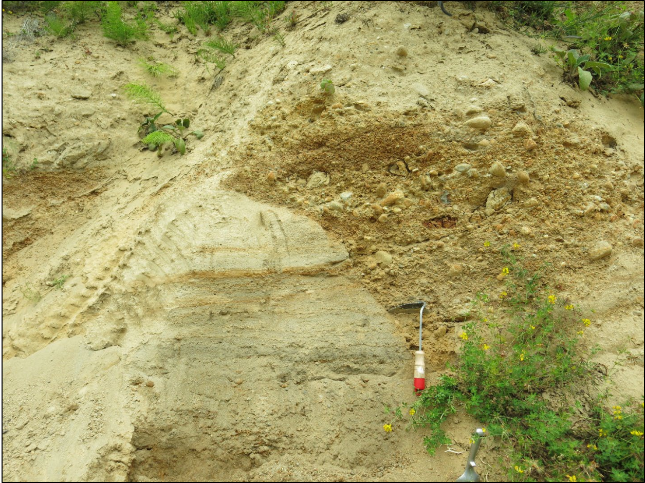
Figure A1-7. Light grey to tan sand with minor pumice layers (left) cut by oxidized sand to cobble deposit (right) at field station 19GW87.1. Scraper is approximately 25 cm long. Unit Qfch, probable fluvial and tidal deposits related to Chehalis River. View to north.
