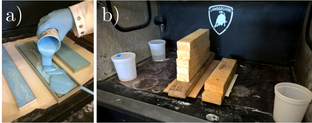
Figure 2.9: Creating Silicone Molds: a) pouring silicone mixture; b) applying pressure while molds cure
