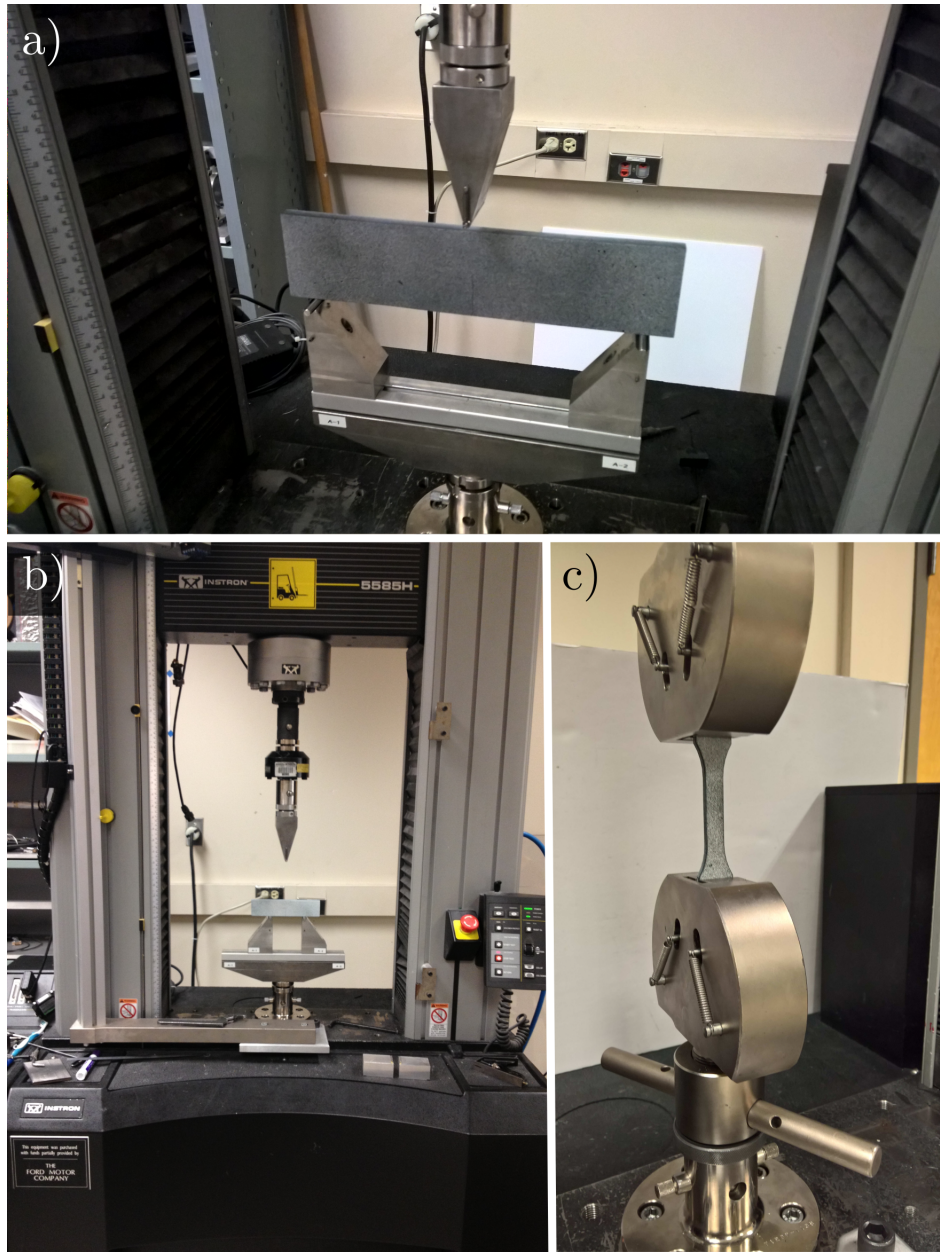
Figure 2.15: Instron Testing Machine: a) detail of SENB setup; b) view of instron machine; c) detail of dogbone setup
