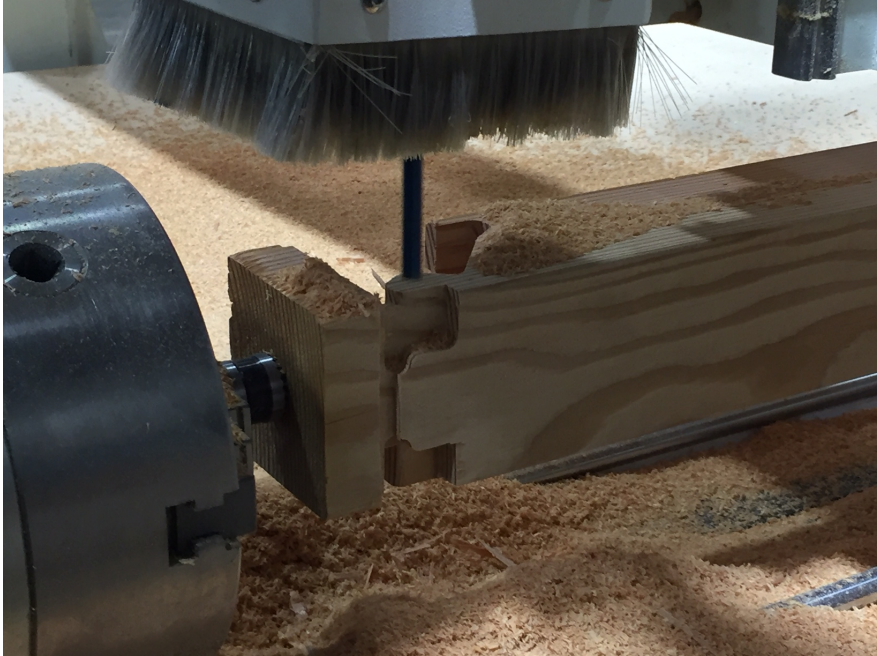
Figure 5.8: Image of 4-axis milling process. A part of the stock was left to continue milling across each of the four axes.
