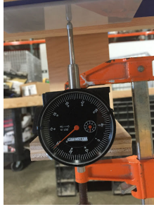
Figure 5.5: The analogue indicator could gather measurements with a precision of up to 30 micrometers.
