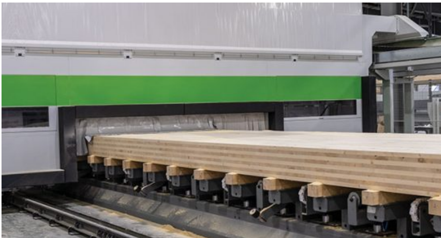
Figure 2.6: View of the CNC machine on a track. These tools can be used for large scale milling for mass timber elements such as CLT and Glulam. (Kalisnekoff, Castlegar, B.C., Canada; 2021)
