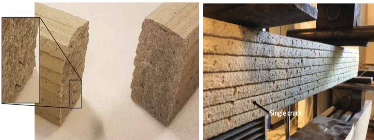
Figure 2.11: Printed beam with embedded reinforcement in 4-point bending (Salet et al., 2018).
