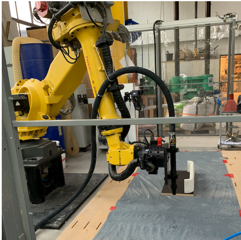
Figure 4.9: Robotic Arm calibration at the Danish Technological Institute (Photo by author).
