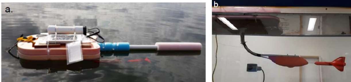
Figure 5.6 (a) Photo of constructed current sensor deployed in field. (b) Bottom view of current sensor displaying the 3D printed propellor mechanism in the flume. (c) Plot showing the relationship between current speed and the proportion of snails with matched radulae (implied residents of the site).
