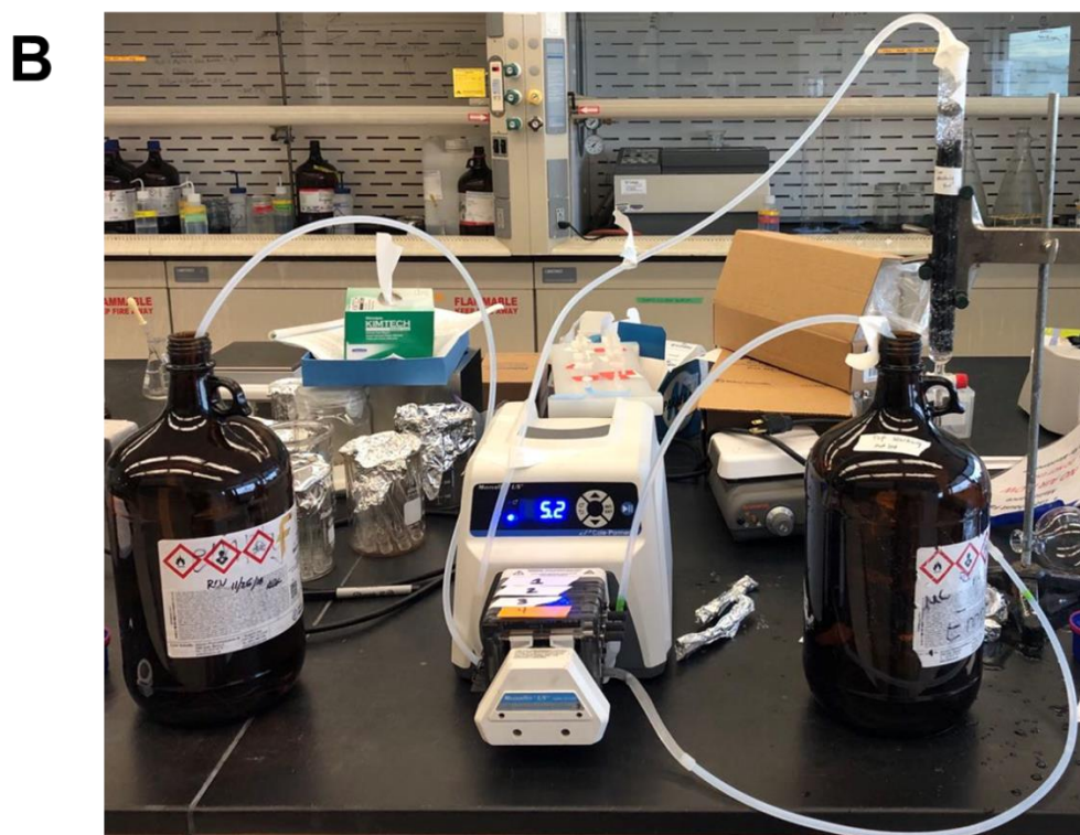
Figure S2.1. The flow-through leaching system setup. (A) Schematic diagram of the setup; and (B) photo of the leaching system setup in the lab.
