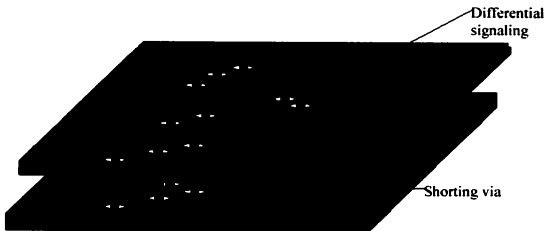
Figure 28: Typical multi-via structure
