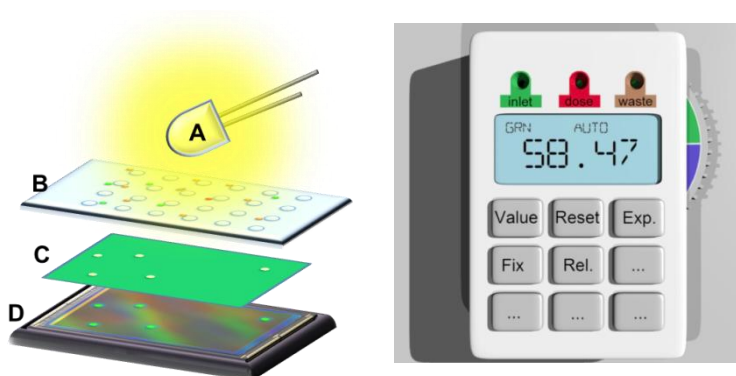
Figure 5-1. Schematic illustrations of Micro Trapping Cytometer. Left: A) fluorescence light source; B) trapping array layer; C) fluorescence filter layer; D) detector layer; Right: Schematic illustration of a hand-held prototype device.
