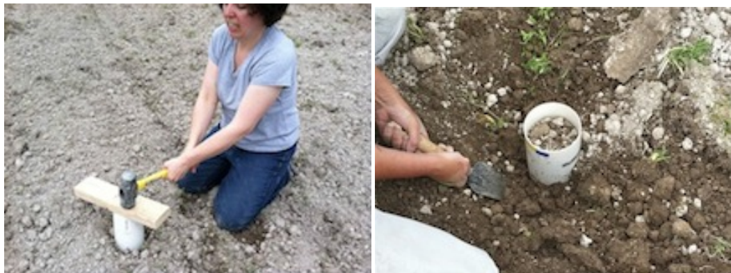
Figures 2.3 and 2.4. Using PVC pipe measuring 10cm in diameter and 30cm in length, columns were hammered directly into the soil and removed intact. This photograph is at the agricultural site where a plow pan was reached at about 7.5cm in soils with a silt-loam texture.
