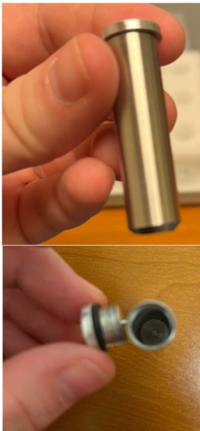
Figure 3.33. Photographs of stainless-steel screw top vial used for vortexing mechanoredox RAFT studies.
