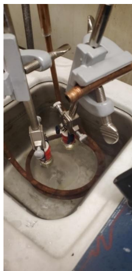
Figure 2.2: Photograph of a typical US-mediated FRP reaction setup. Reaction vials are immersed into the water bath via clamps and a coiled copper tube connected to a recirculating chiller is used for temperature control of the bath.
