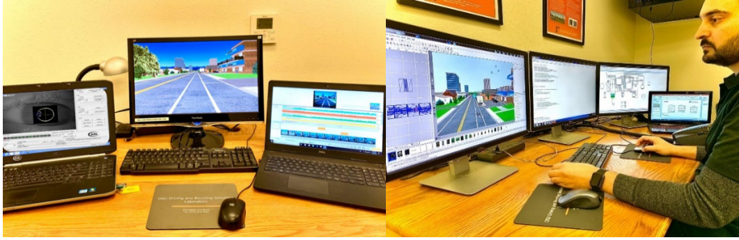
Figure 6.2 Operator workstation for the bicycling simulator. Left: Real-time monitoring of the simulated environment. Right: A researcher designing an experiment in SimCreator.
