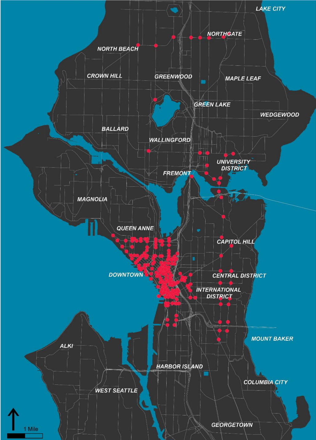
Caption: This map shows the locations of the Acyclica sensors in corridors throughout the City of Seattle. There are currently over 200 sensors in major arterial corridors in the city, and SDOT is interested in expanding the program. Program managers believe that this is one of the most successful traffic mitigation technologies available.
