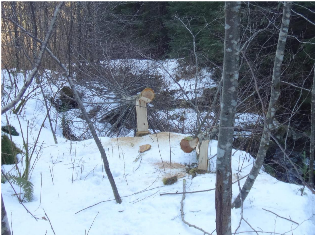
Figure 8. Cross-sections are removed from the base of the largest alders growing on a terrace deposit. The annual rings of the alder were examined to determine the tree age and infer the year the terrace formed.
