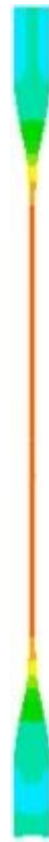
Figure 7-5: Deformed finite element model during creep tests at creep stress of 5.6 MPa, 31% of the ultimate tensile strength.
