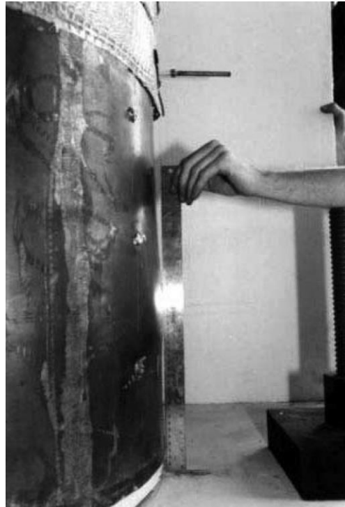
Figure 3.11 Bulging of the steel confining jacket (from Hewes and Priestly 2002)
