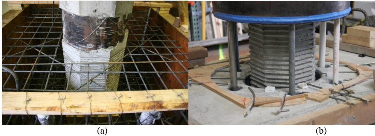
Figure 4.2 Precast connections. (a) “Wet socket” connection. (b) “Hybrid-bar-socket” connection. (Note the photos show the connections in the orientation used for testing).
