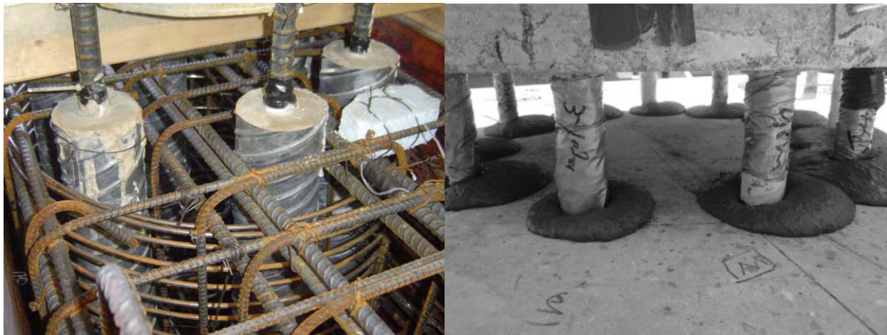
Figure 2.4: Grouted bar connections (from Pang et al. 2010 and Tazarv and Saiidi 2014, respectively).
