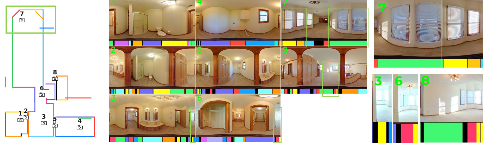
Figure 3.11: Failure case caused by incorrect MOIS wall-instance prediction, where MvFFN fails to distinguish different wall instances across views.
