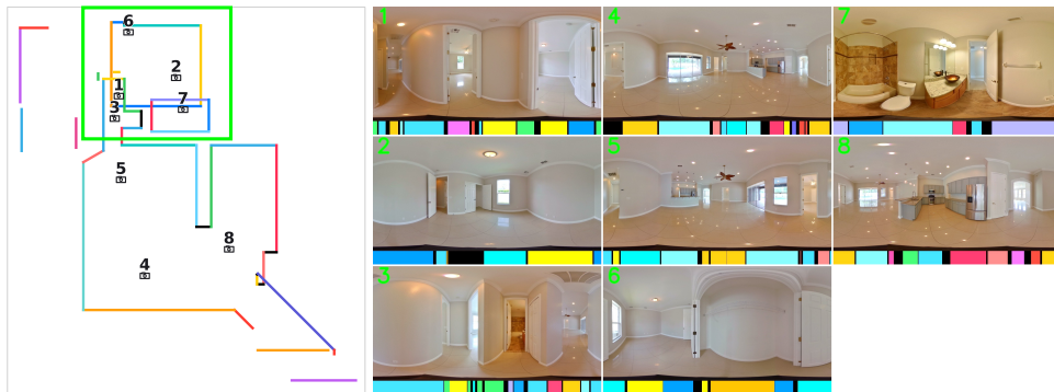
Figure 3.12: Failure case caused by geometric errors in the initial MvFFN predictions, where inaccurate poses and point maps lead to distorted layout geometry.
