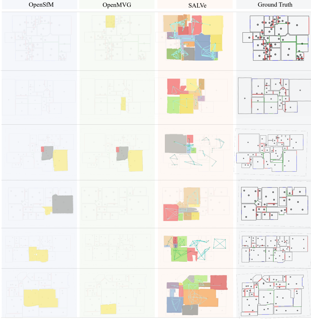
Figure 2.7: Qualitative comparison of floor-plan reconstruction. Columns show OpenSfM , OpenMVG , SALVe , and ground truth, all overlaid on the ground-truth floor plan. Colored regions indicate reconstructed coverage, showing that SALVe recovers more complete layouts. Colored lines denote doors , openings , and windows ; cyan edges indicate verified W/D/O alignments.
