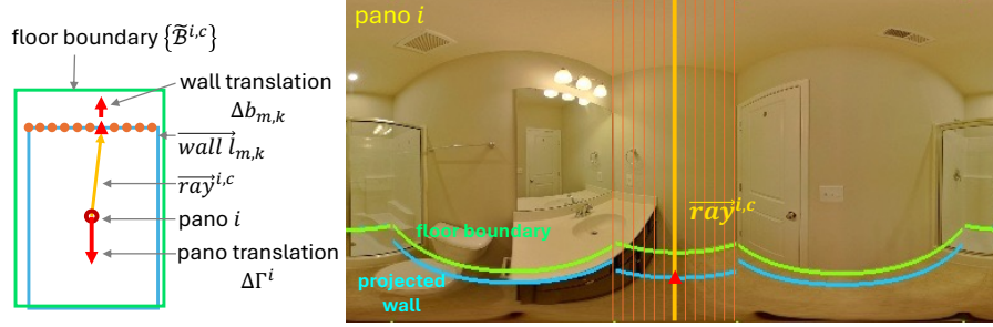
Figure 4.4: Column-wise planar BA module. Positional adjustment for walls and cameras are computed for each image column. At each column, the associated wall l_{m,k} is projected with the current camera pose E^i . The adjustments are computed by comparing the projected point to the floor boundary \tilde{B}^{i,c} value. The dense per-column adjustments are estimated in parallel with our BA layer implementation.
