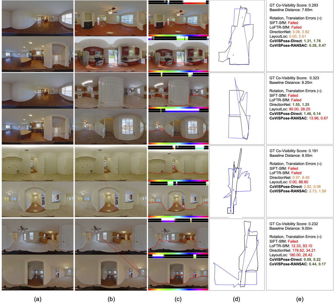
Figure 3.3: Qualitative results on ZInD. (a) SIFT feature point inliers generated by 2-view SfM with OpenMVG [42], (b) LoFTR [67] feature point inliers generated by the same solver as (a), (c) CoVisPose prediction, (d) predicted floor-wall boundaries for Panorama 1 and Panorama 2 aligned by CoVisPose direct regression. (e) Pose errors for each method. Color scheme corresponds to maximum of rotation and translation errors: Failure to recover pose or error > 10^\circ , error in [2.5^\circ, 10^\circ] , error < 2.5^\circ .
