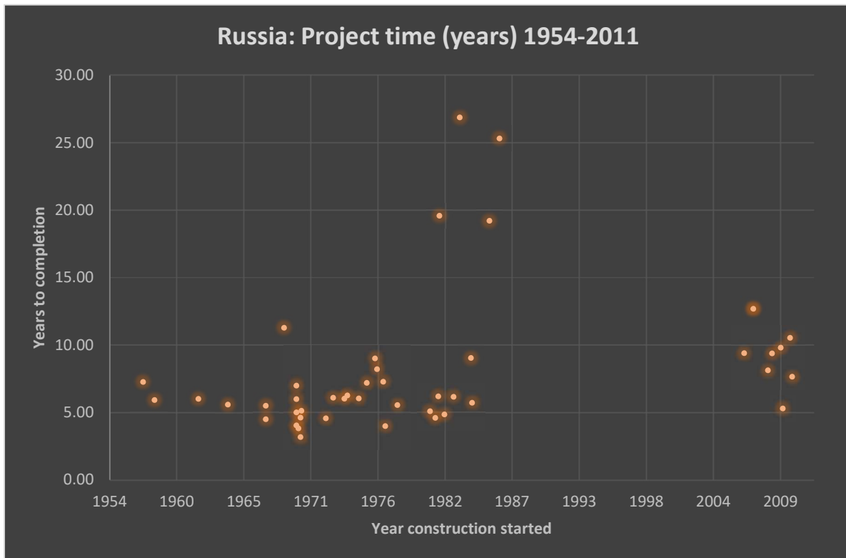
Figure 9-- Construction times for reactors within Russia. Source: Data from IAEA PRIS database. Author's own graph.
