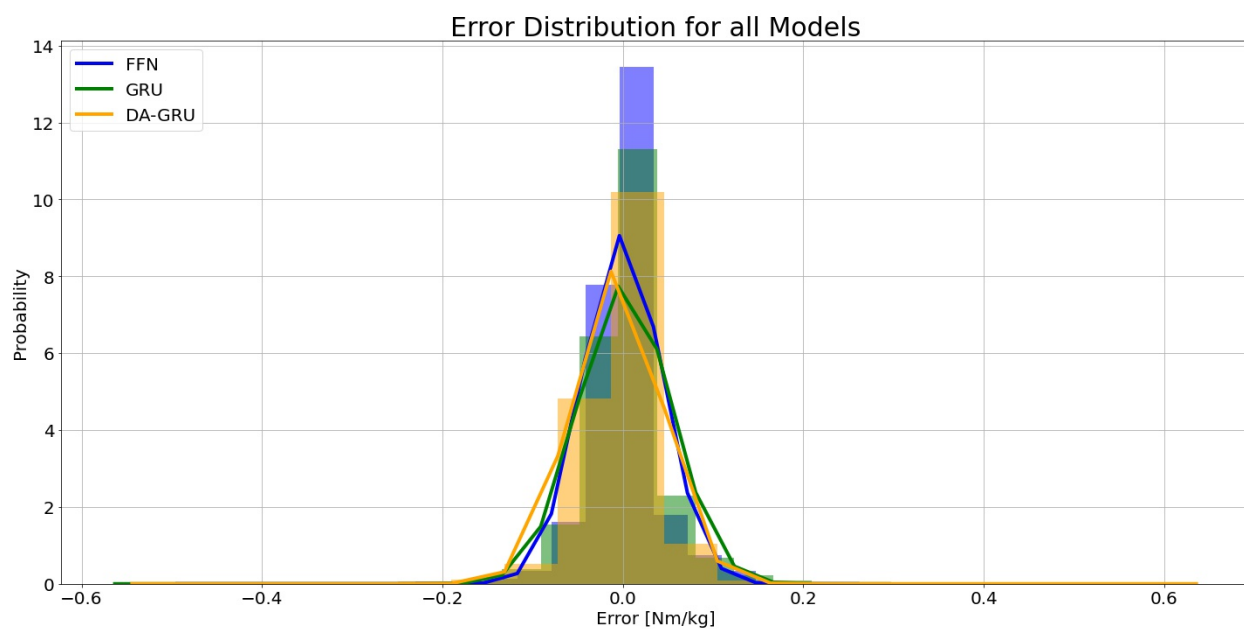
Figure H.1: Prediction error histogram for all DNN models across all test time series data.
