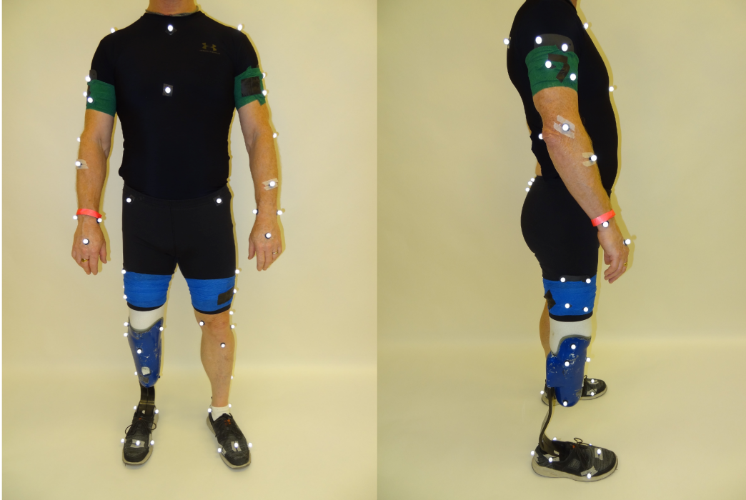
Figure 5.4: Modified plug-in gait reflective marker set placed on subject A01.
