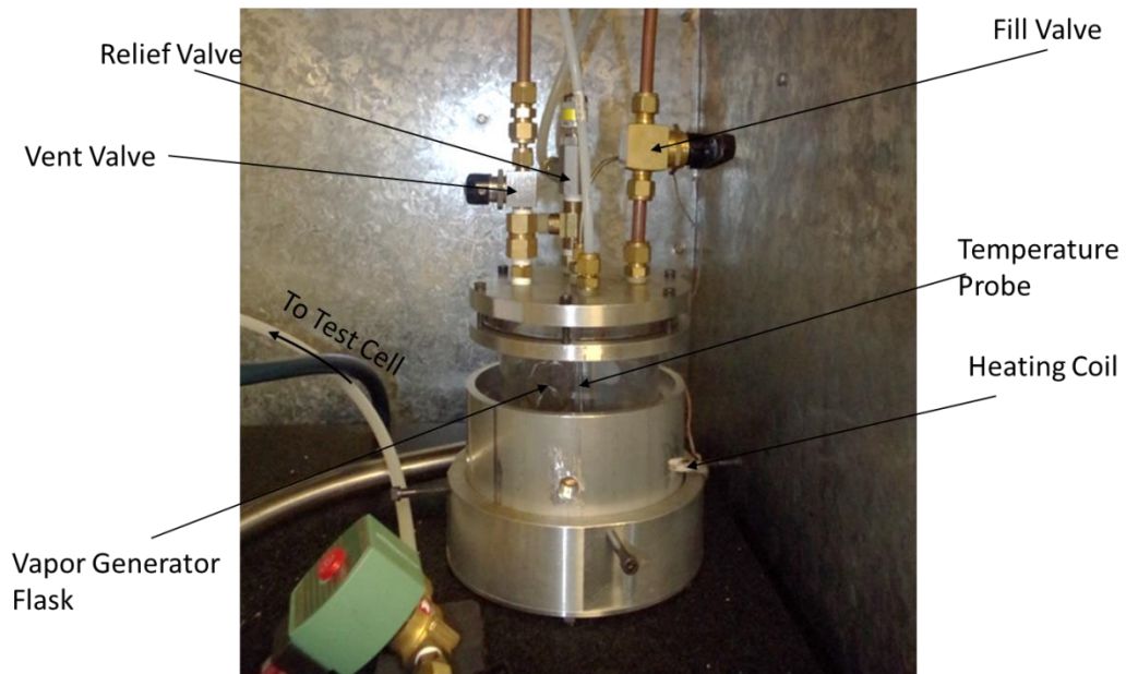
Figure 2.2. Vapor generator sub-system (diameter approximately 15 cm (6 inches)).
