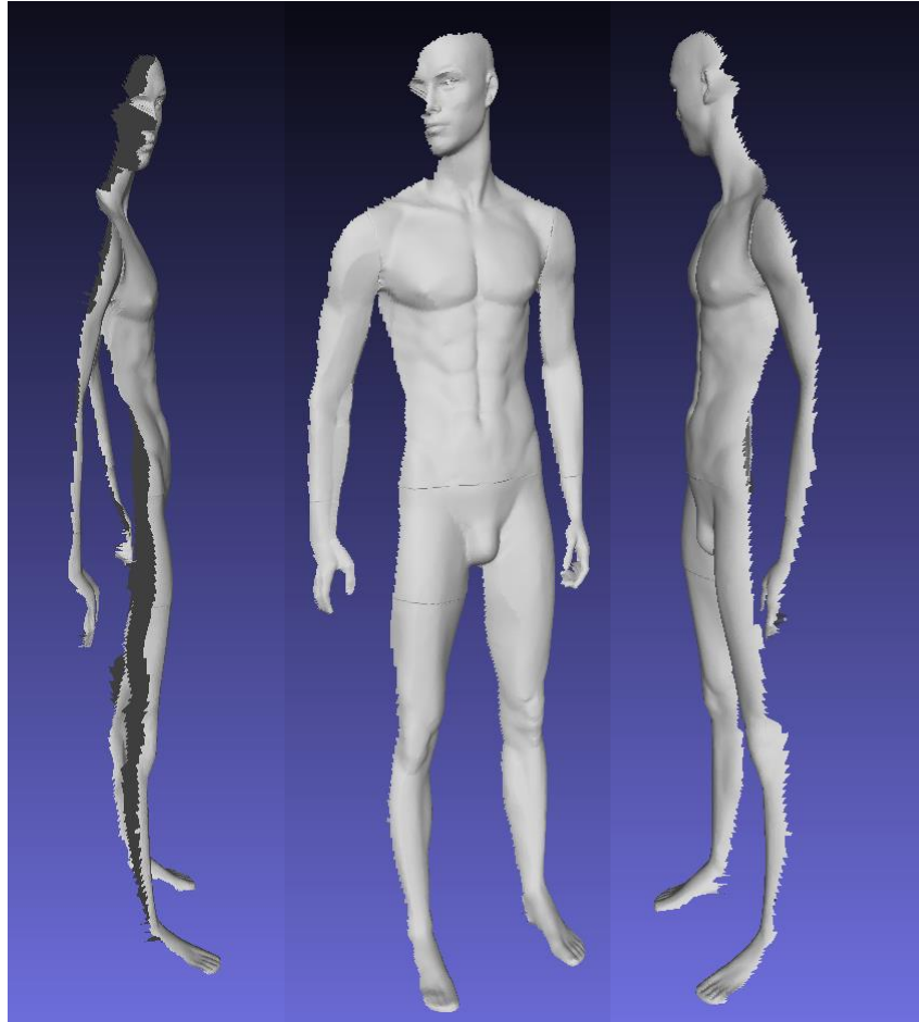
Figure 3.10. Multiple views of a reconstruction of a 2m tall mannequin with sharply detailed surface geometry. The mannequin was more specular than human skin due to its plastic material.
