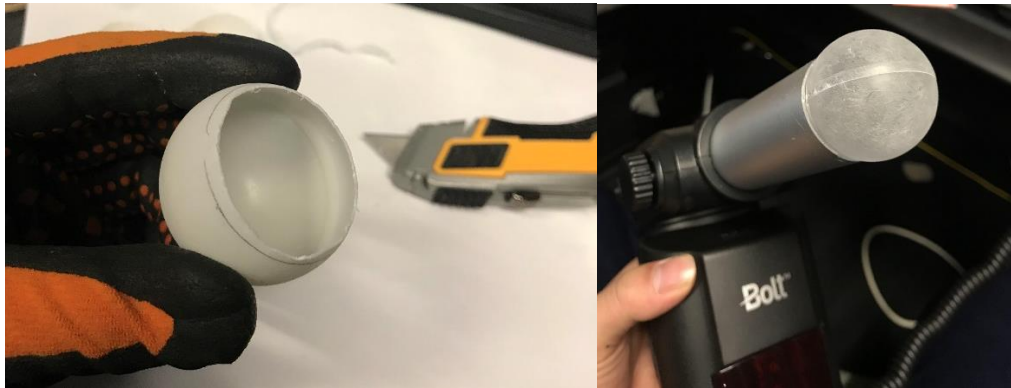
Figure 3.4. Left: Spherical diffuser made by cutting out one end of a ping-pong ball. Removing transmissive surfaces kept the light output higher. Right: diffuser made by sanding the exposed portion of a clear plastic ball into a frosted appearance.
