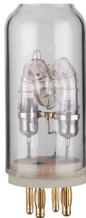
Figure 3.3. Bolt VB-22 flash bulb. The coiled emitter and nonuniform glass refraction nullify the assumption of a point light model in photometric stereo. A uniform isotropic diffuser is necessary to filter this light source into a point-like distribution.
