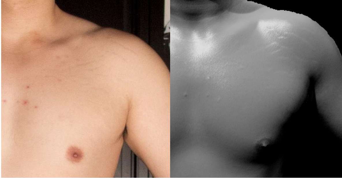
Figure 3.8. Close up of chest area on one of the photos in the photometric stereo sequence (left) compared to the reconstruction (right) with no textures present. Very small-scale surface deformations such as stretch marks were captured as geometry in the 3D reconstruction. The primary benefit of photometric stereo is the ability to capture pixel-resolution detail as surface geometry.
