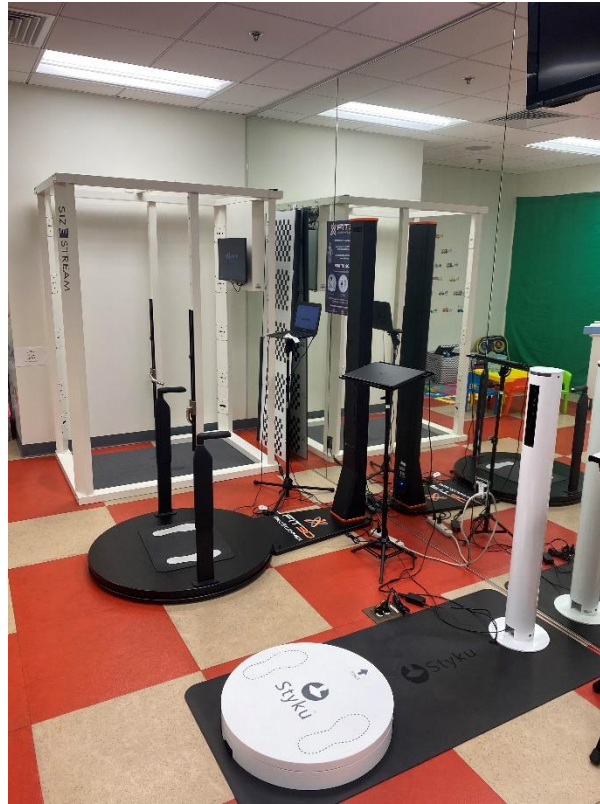
Figure 1.1 Three 3D optical (3DO) scanners used for data collection in this thesis. From back to front: SizeStream SS20, Fit3D Proscanner 4.x, Styku S100.
