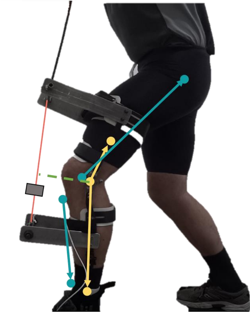
Figure 13: Definitions for vectors used in stiffness calculations. Shank vector was shifted anteriorly in this image for clarity.
