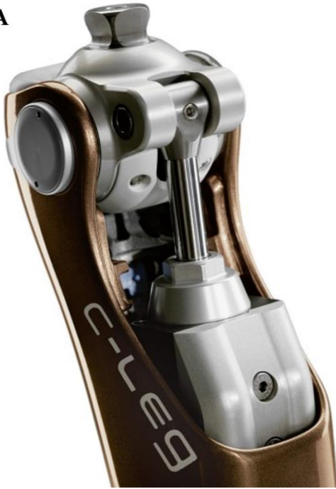
Figure 2: Two examples of modern prosthetic devices. A) The quasi-passive C-Leg from Ottobock changes the state of a hydraulic valve to change knee damping during gait. B) The Ottobock Empower is the only active prosthetic foot on the market. (Ottobock, Duderstadt, Germany)
