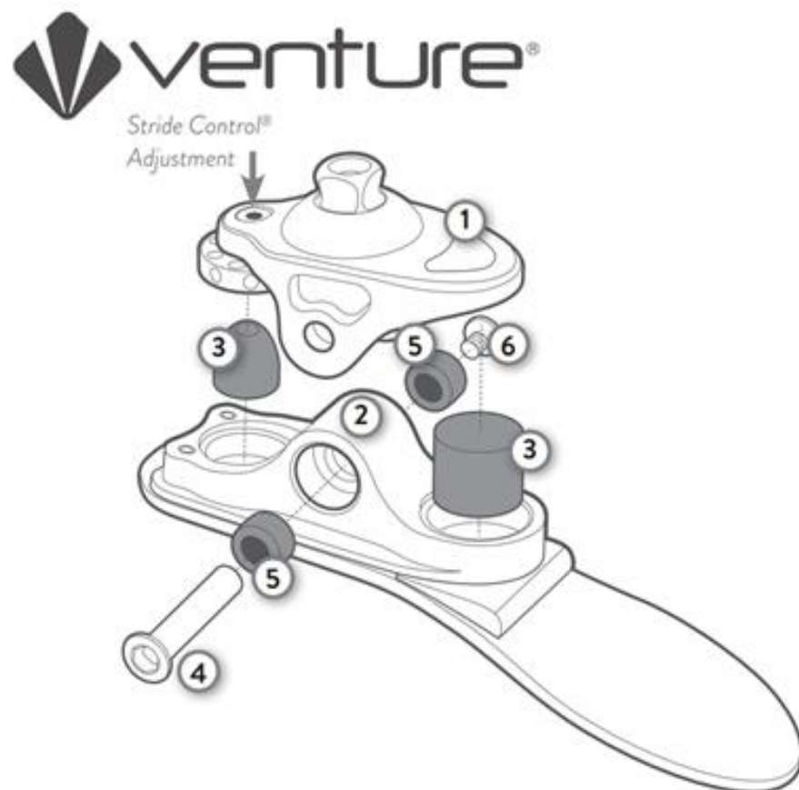
Figure 7: Exploded view of the College Park Venture Foot. 1. Top 'ankle bone.' 2. Bottom 'ankle bone.' 3. Bumpers. 4. Axial pin. 5. Ankle Bushings. 6. Axial Pin Screw. (College Park Industries, Warren, MI, USA)
