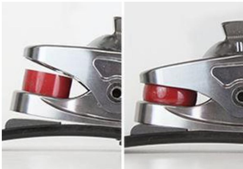
Figure 34: Venture Foot by College Park. The left frame shows the foot in an unloaded state. Note the gap between the carbon fiber keel and metal ankle bone. The right frame shows the foot loaded in dorsiflexion, and the gap has closed. (College Park Industries, Warren, MI)
