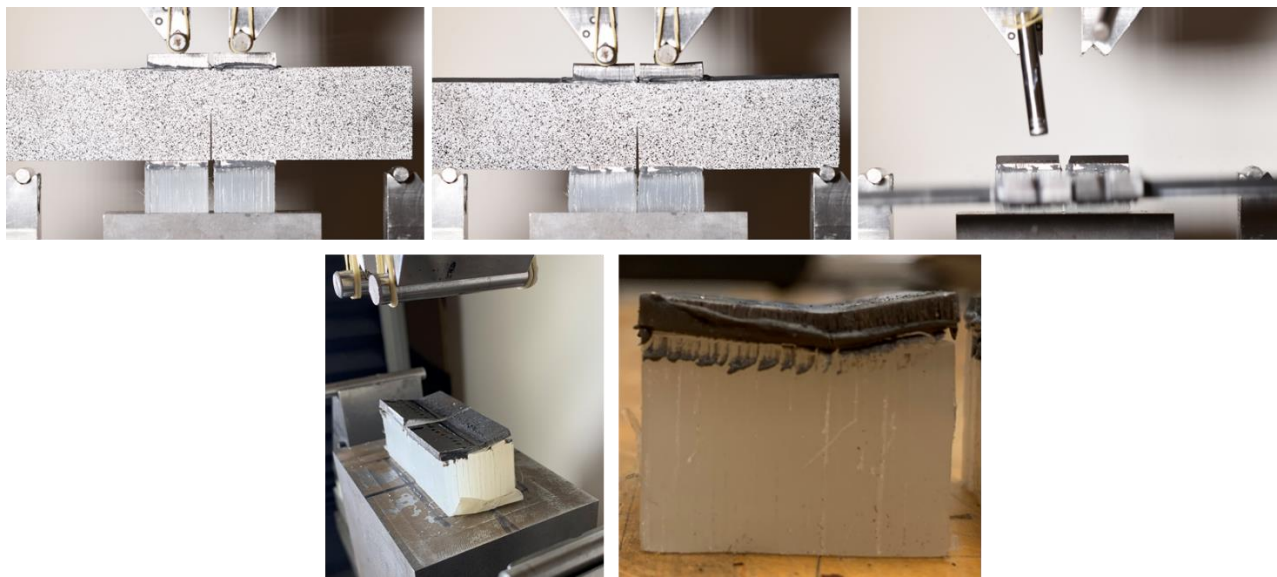
Figure 3.4 Second design iteration failures when attempting to apply crack parallel compression (top) test specimen toppling prior to fracture (bottom) structural instability in polypropylene pads that causes toppling.
