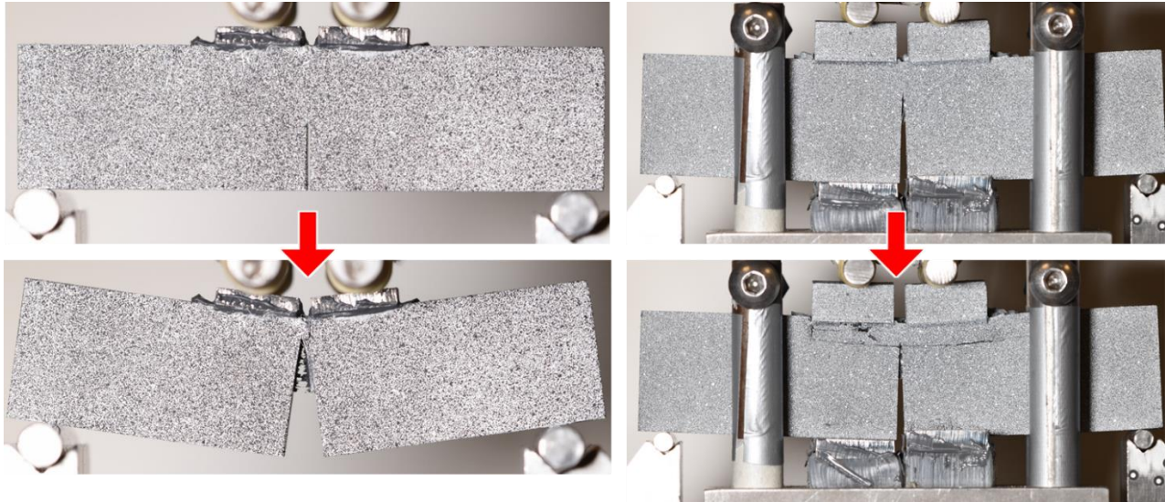
Figure 3.14 Representative images of the post peak behavior differences for a Gap Test without and with crack parallel compression. (left) \xi = 0 small panel exhibiting stable crack propagation (right) \xi = 0.44 medium panel exhibiting transverse fracture after initially unstable crack propagation.
