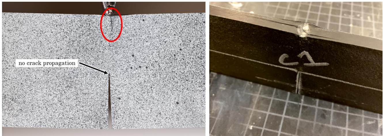
Figure 3.1 Delamination failures that occur due to stress concentrations in the initial Gap Test design.
