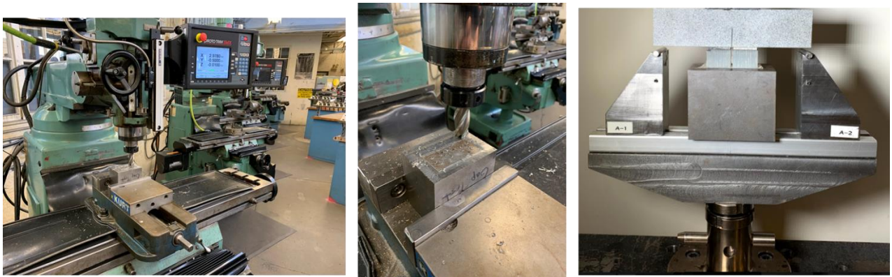
Figure 2.8 In process machining and final images of the first test fixture design for composite Gap Testing.
