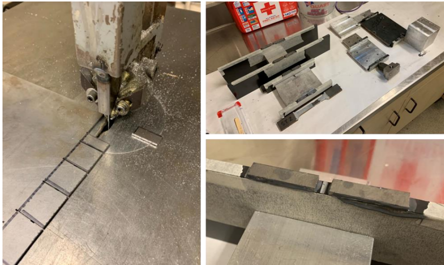
Figure 3.2 Additional test specimen preparation required to include steel caul sheets with a 4PB loading condition.
