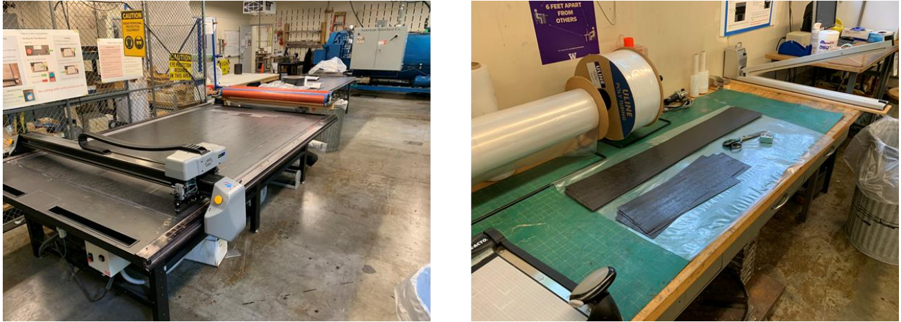
Figure 2.9 (left) CNC ply cutter cutting pre-preg composite into the desired size, shape, and quantity of plies (right) ply kit containing the necessary plies for the composite part.
