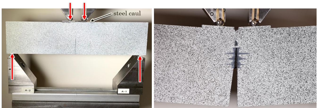
Figure 3.3 Second design iteration used to execute the Gap Test on composites.
