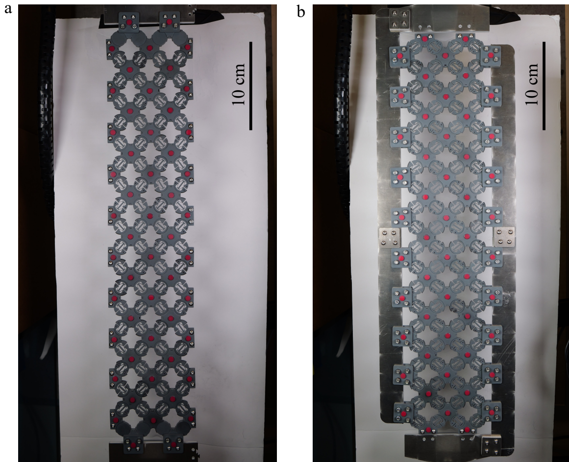
Figure 3.4: The 4 \times 18 array under tensile loading (a) and shear loading (b). Red markers are used for optical tracking to extract local strain information in the array.
