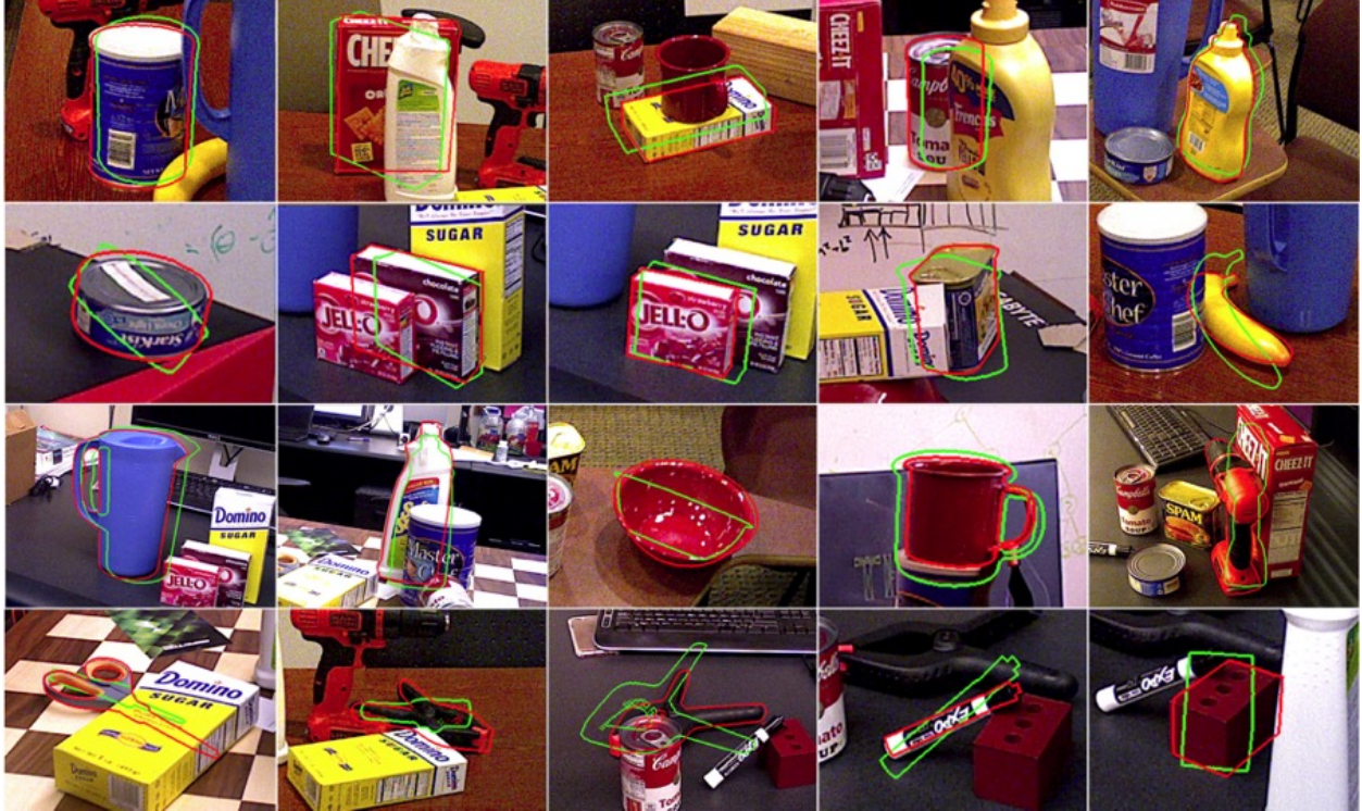
Figure 2.10: Examples of refined poses on the YCB-Video dataset which use results from PoseCNN [Xiang et al., 2018] as initial poses. The green and red lines represent the silhouettes of the initial estimates and our refined poses, respectively.
