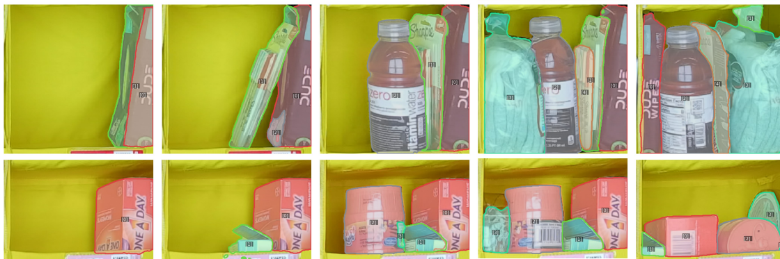
Figure 3.4: Visualized results for the shelf environment. Masks with the same color and index are associated and predicted as the same object by the network.
