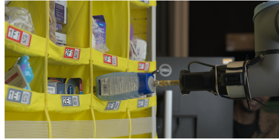
Figure 3.1: A densely packed shelf environment. The shelf holds objects from a wide array of categories. During the stowing process, a human operator may obscure the camera’s view and rearrange the objects within the bin. The robot’s task is to pick a specific object as directed by the given order index of the object’s placement in the bin.
