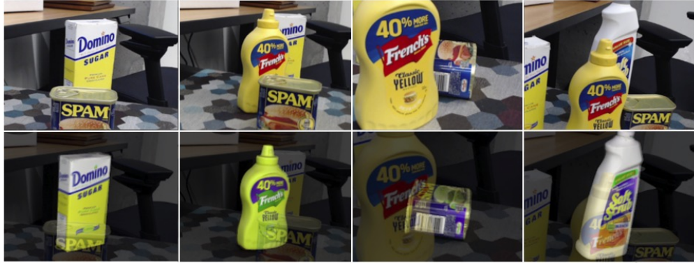
Figure 2.11: Examples on tracking in the real world, using the same network as in Table. 2.10 and no prior knowledge about focal length. The first row shows the images captured with a webcam and the second row renders the object onto the image based on the estimated pose.
