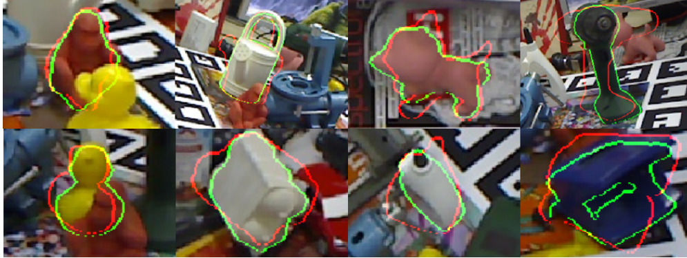
Figure 2.9: Examples of refined poses on the Occlusion LILNEMOD dataset using the results from PoseCNN [Xiang et al., 2018] as initial poses. The red and green lines represent the silhouettes of the initial estimates and our refined poses, respectively.
