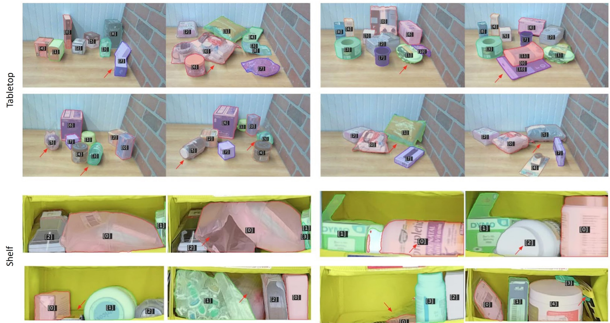
Figure A.5: Failure Cases Illustrated. In the Tabletop settings (top 2 rows), we observe under-segmentation (top left), over-segmentation (top right), mismatch (bottom left), and mistrack (bottom right). In the Shelf settings (bottom two rows), the failures include a combination of under-segmentation and failure to detect new objects (top left), failure to track and mismatch (top right), failure to detect (bottom left), and failure to segment (bottom right).
