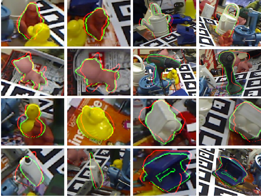
Figure 2.7: Some pose refinement results on the Occlusion LINEMOD dataset. The red and green lines represent the edges of 3D model projected from the initial poses and our refined poses respectively.
