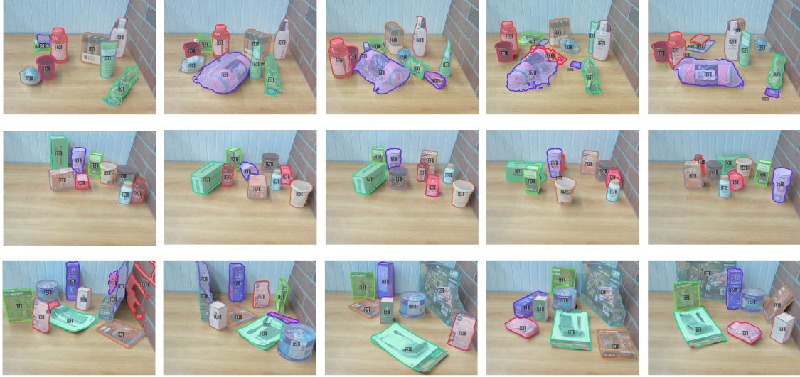
Figure 3.5: Visualized results for the table environment. Masks with the same color and index are associated and predicted as the same object by the network.
