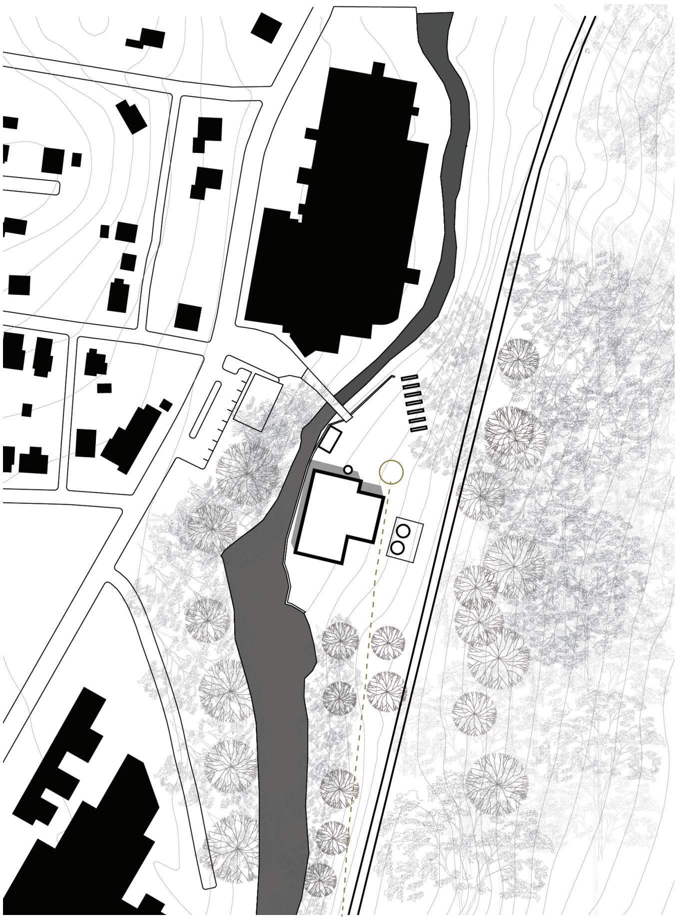
30 22. site plan of existing steam plant showing bridge, trestles, building, smokestack, trailhead and coal silos
