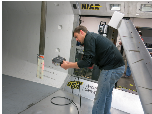
Figure A.4: Obtaining precise measurements of the location of the tips with respect to the laser locator.
