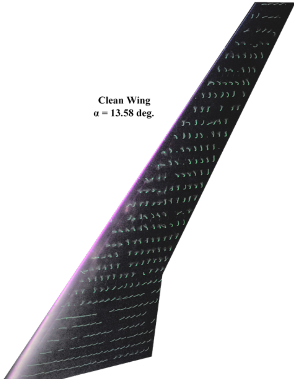
Figure 4.8: Mini-tuft imagery for the clean wing for \alpha = 13.58^\circ , Re = 1.6 \times 10^6 , M = 0.17 .
