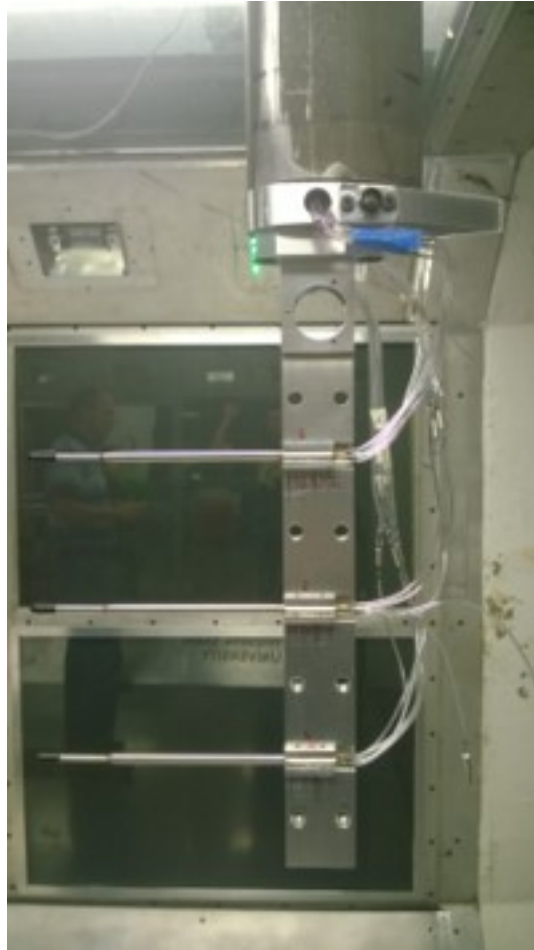
Figure 3.6: An image of the wake survey probe array in the tunnel. Note that this image does not show the aerodynamic fairing. Adapted from Lum [41].
