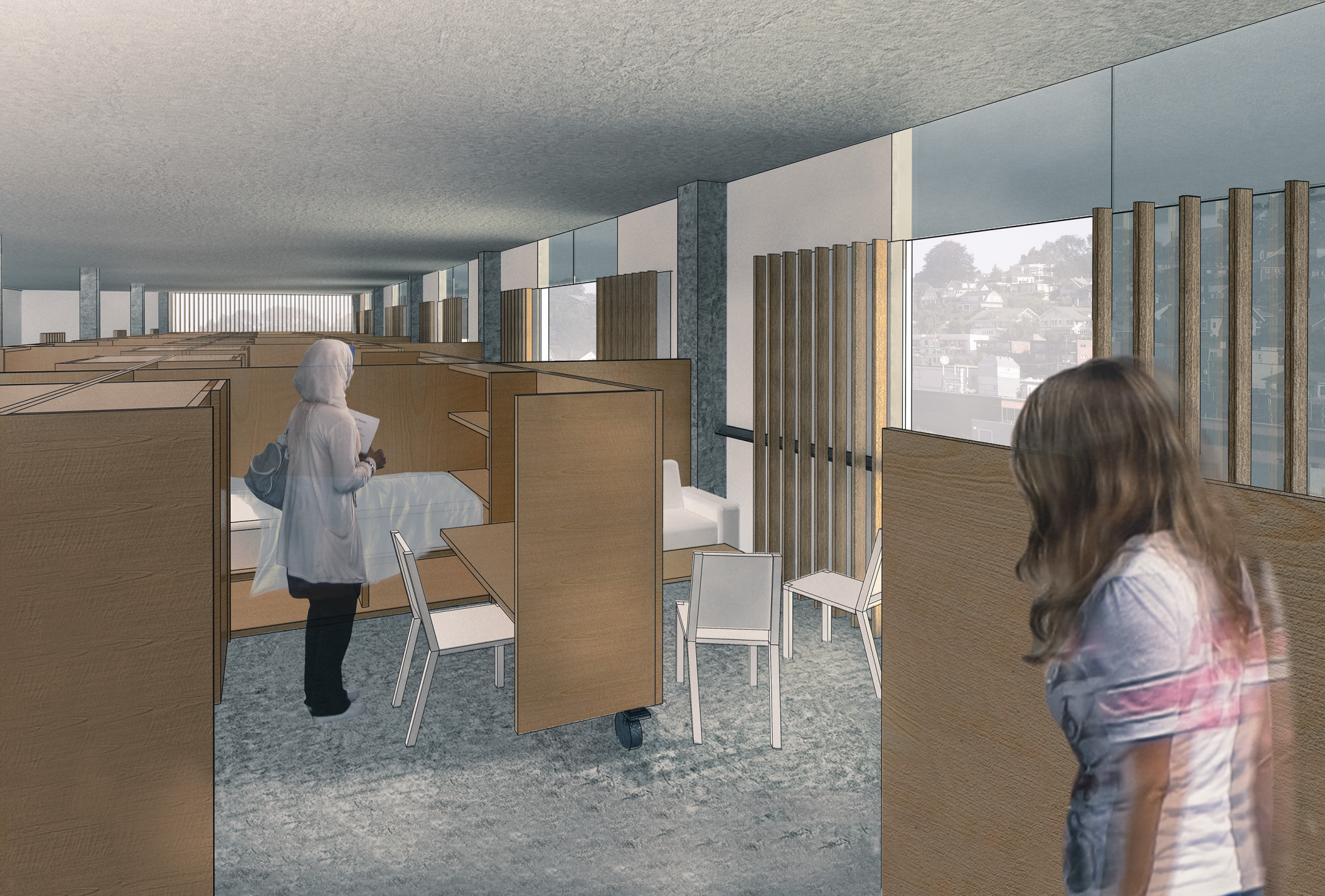
Figure 64: These partially enclosed plywood units, designed in 4 foot dimensions to conserve materials and cut costs, provide some degree of privacy while allowing many residents to be supervised by few members of staff. Sliding wooden screens allow for customization of the living space, fostering a sense of personal ownership despite not being completely enclosed. These vertical wood screens also establish an architectural relationship with the rest of the living units on site.
