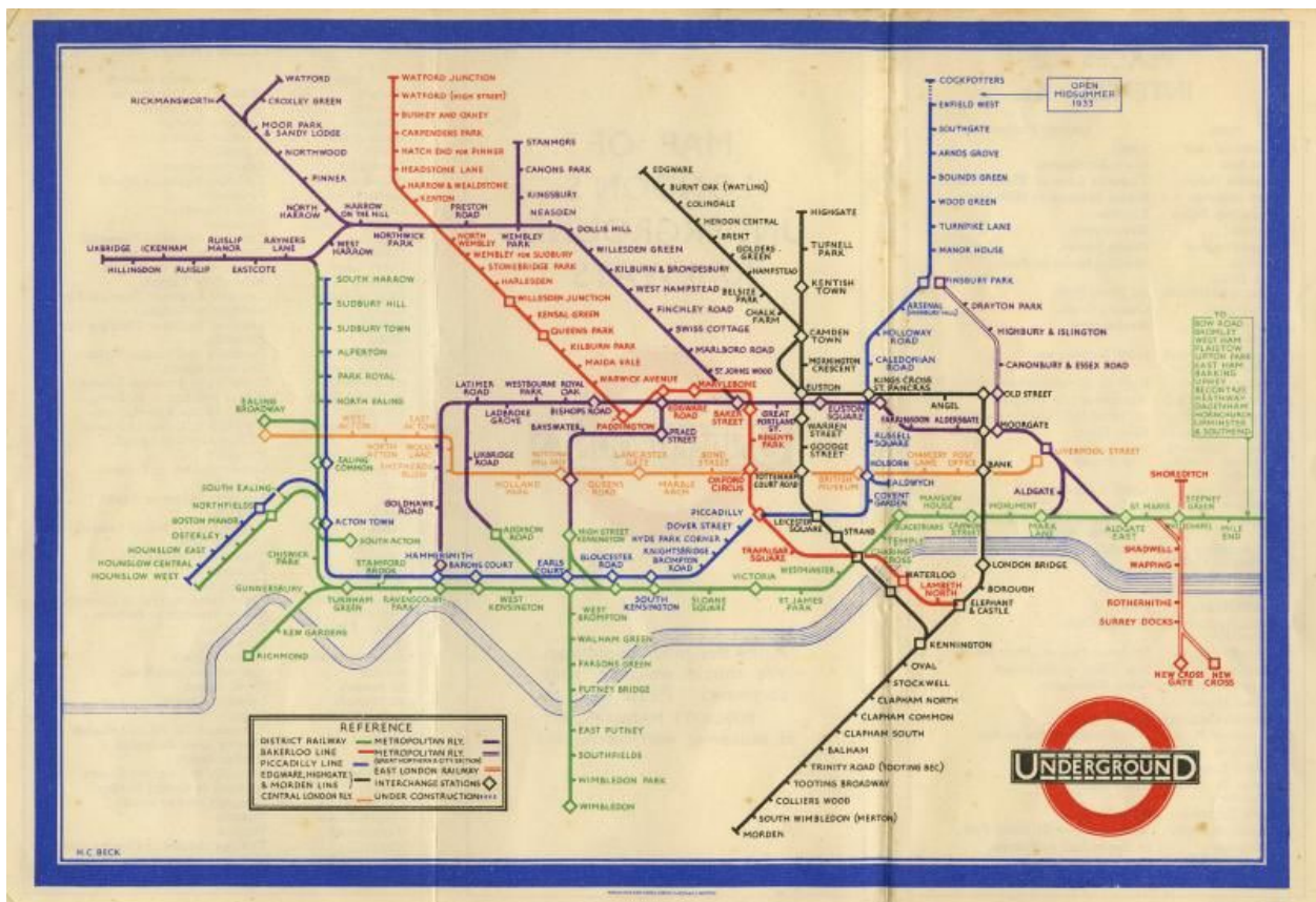
(Figure 9) Henry Beck map 1933. The first pocket edition of the diagrammatic style of Underground map designed by Henry C Beck. It highlights the use of 45-degree angles and diamonds to illustrate interchange stations.
