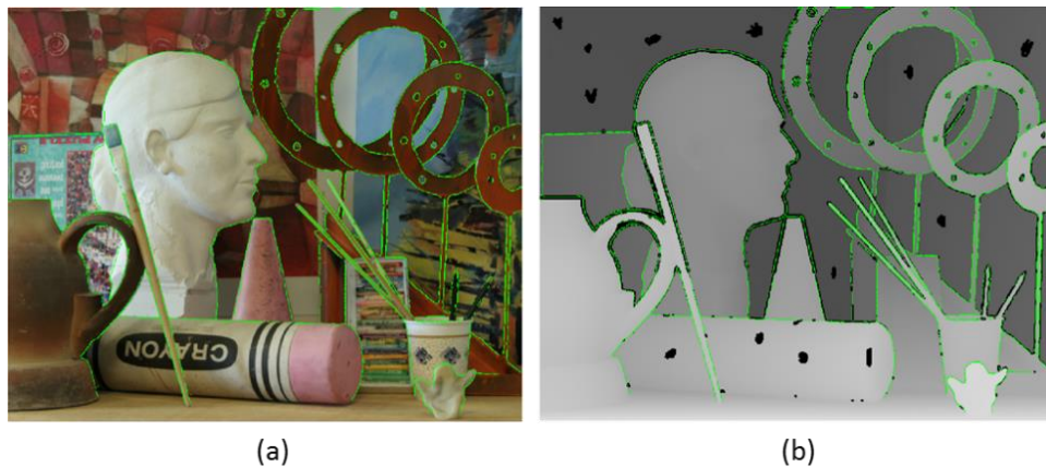
Figure 4-5. Depth edges E from Equation (4.7) overlaid on the color image (a) and on the noisy input depth image (b).
