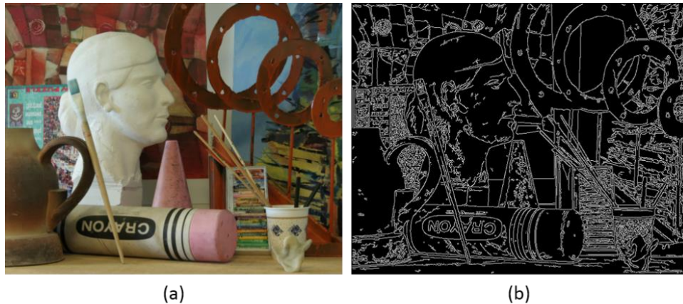
Figure 4-3. (a) Input color image (b) Edges extracted from the color image using the adaptive Canny edge detection
