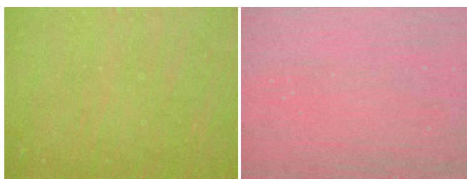
Figure 2.47: Surface quality of sintered PZT on low porous bottom electrode. Thin films are derived from fresh sol (left) and long term aged sol (right) after open air dry.
