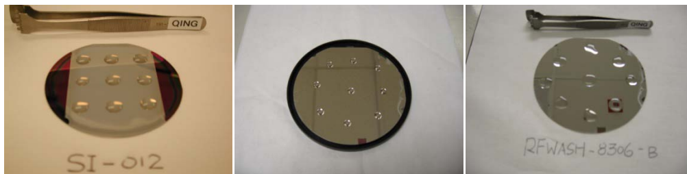
Figure 2.52: Wettability test. From left to right are contact angles of liquid droplets on an annealed wafer without chemical treatment, an unannealed wafer without chemical treatment, and same wafer but with chemical treatment, respectively.
