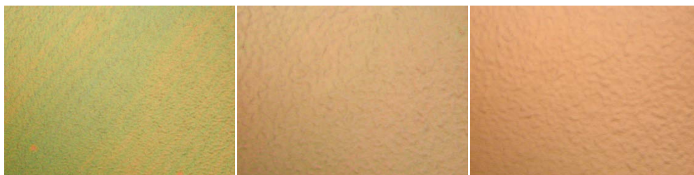
Figure 2.36: Thin-film PZT bumps and dimples inspections on wafer SI-056 at spot 13. Pictures from left to right represent surface non-uniformities on 1 st , 2 nd , and 3 rd layers, respectively.
