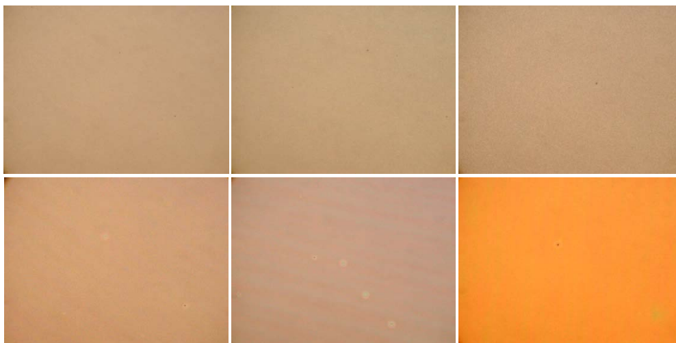
Figure 2.38: Thin-film PZT black dots inspections on 1 st layer of wafer SI-207. Columns from left to right represent inspection spot 11, 21, and 32 respectively. Upper and bottom rows are inspections before and after film sintering.
