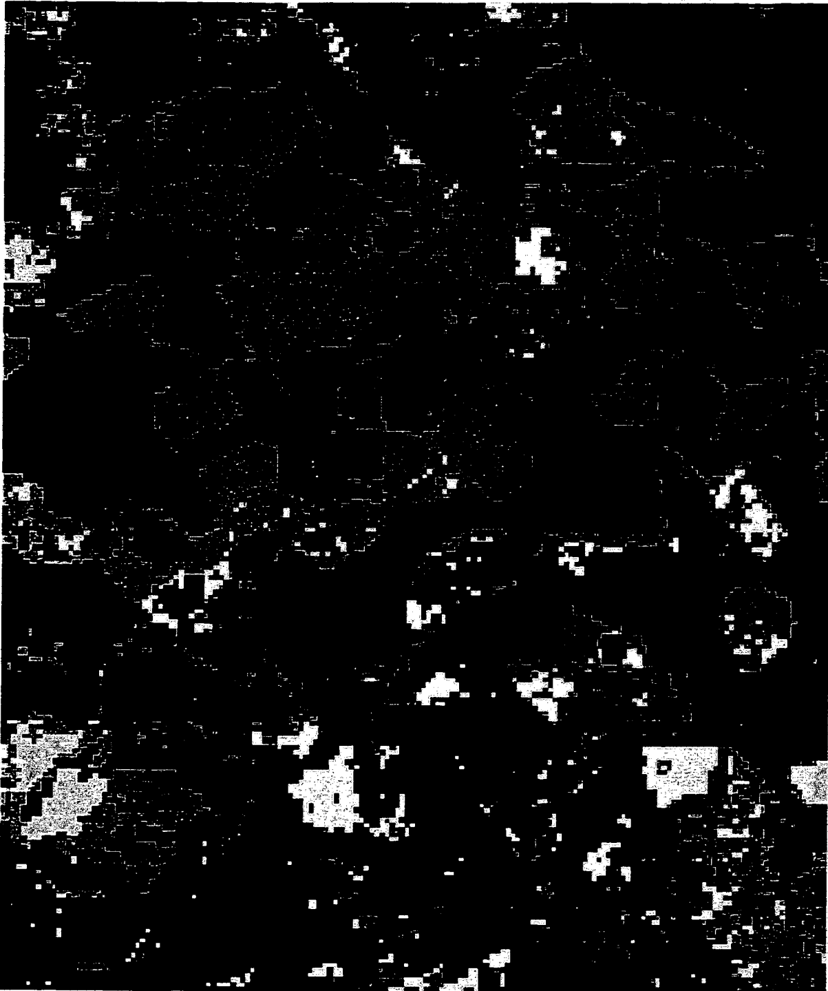
Figure 7.43: ML estimate: July image; data preprocessed for topographic correction using SCS model; low slope training stands.
