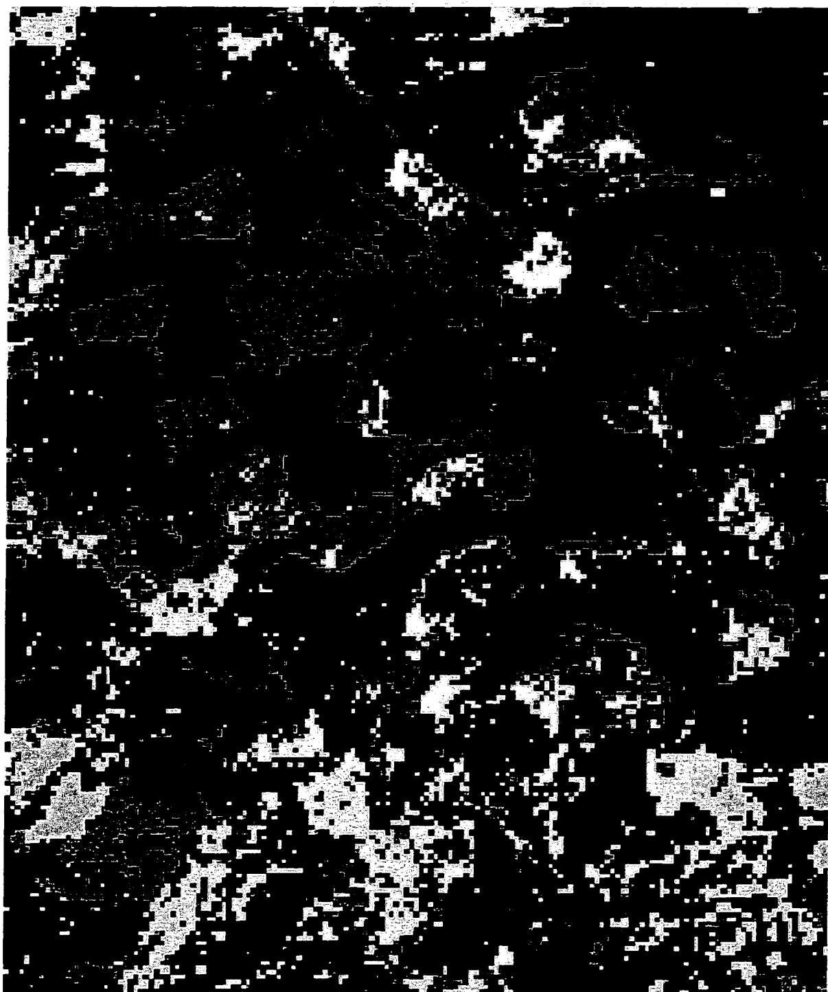
Figure 7.44: ML estimate: August image; data preprocessed for topographic correction using SCS model; low slope training stands.
