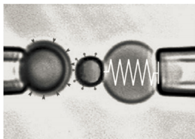
Figure 3: Picture of a biomembrane force probe. The stiffness of a red blood cell is controlled using aspiration pressure. By determining the elongation of the red blood cell, the force between the two beads can be determined. Figure taken directly from Gourier et al., [16].
