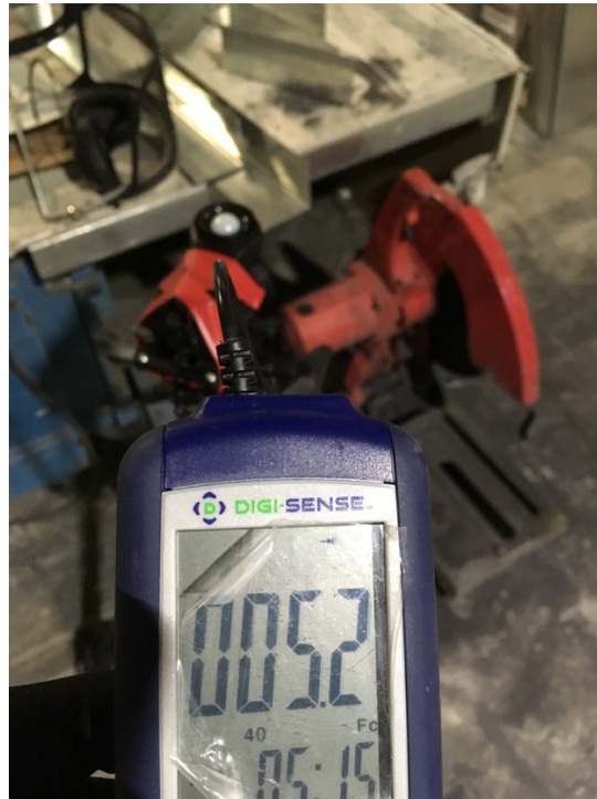
Figure 29: Meter Reading Near Chop Saw Work Station
