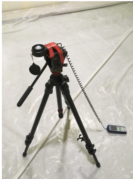
Figure 28: Light Meter Set Up
