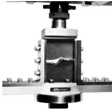
Figure 8. Compression-After-Impact Failed Specimen (Instron, Inc.)
