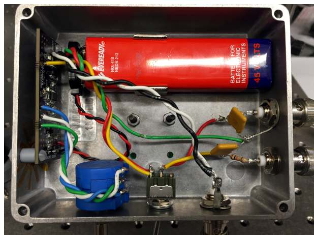
Figure 2.15: Picture of amplified photodiode internals. Note that the 45V battery has been replaced with a 45V power supply.
