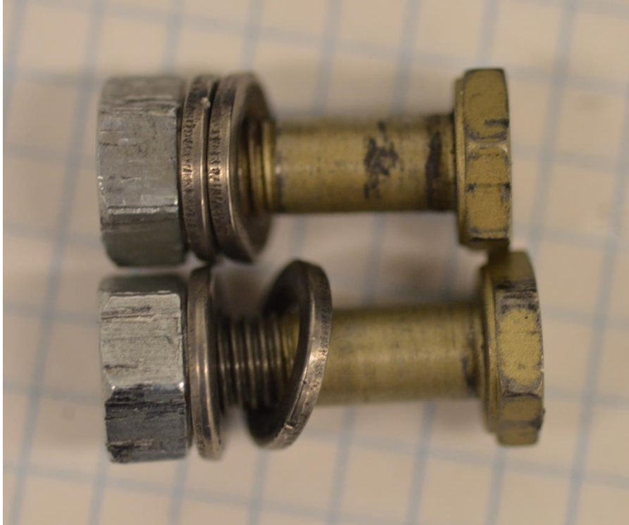
Figure 28: Comparison of fastener shank before (below) and after (above) testing.
