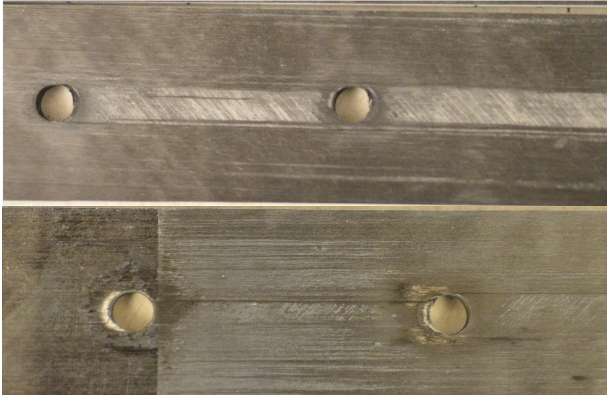
Figure 47: Comparison of Quasi-Static and Fatigue Specimen interfaces
