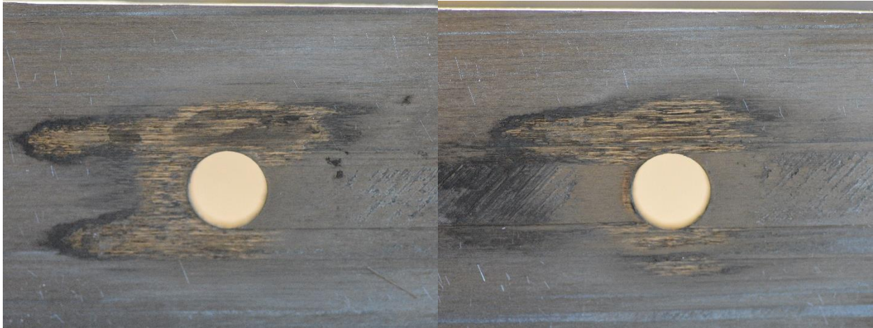
Figure 48: 50% Zero fatigue interface and hole damage, direction of propagation is left to right
