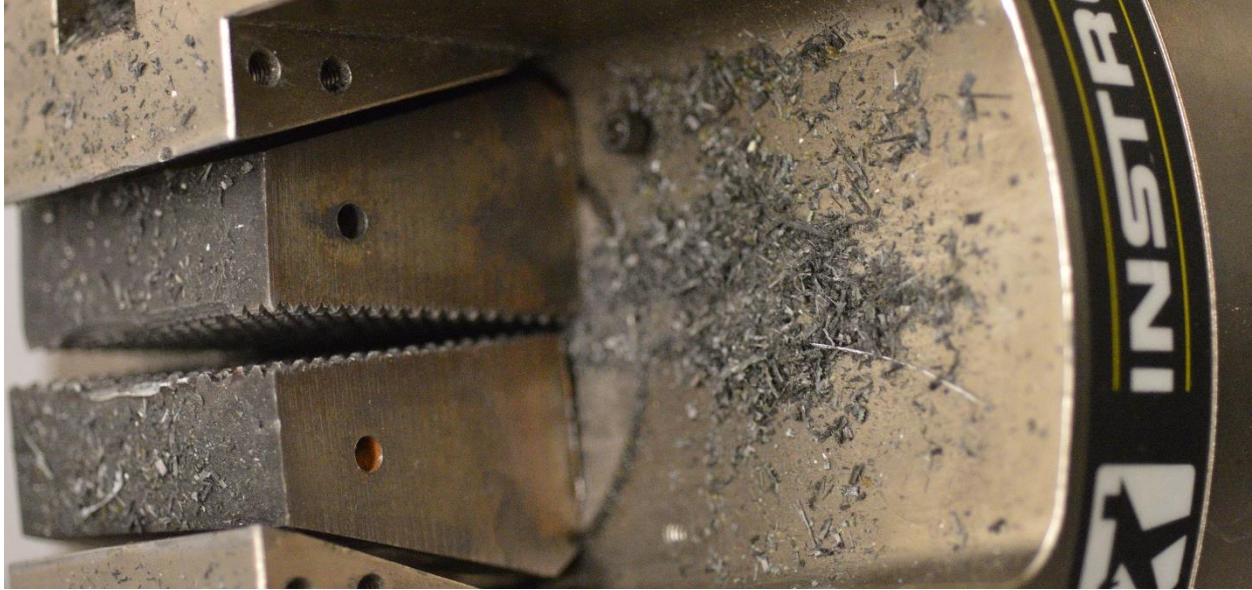
Figure 46: Carbon dust buildup due to cyclic loading, buildup from 3 tests
