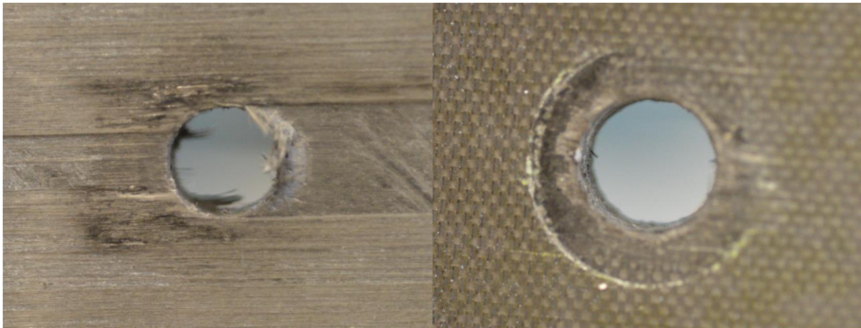
Figure 69: Hole damage interface (left) and underneath washer (right) after fatigue testing
