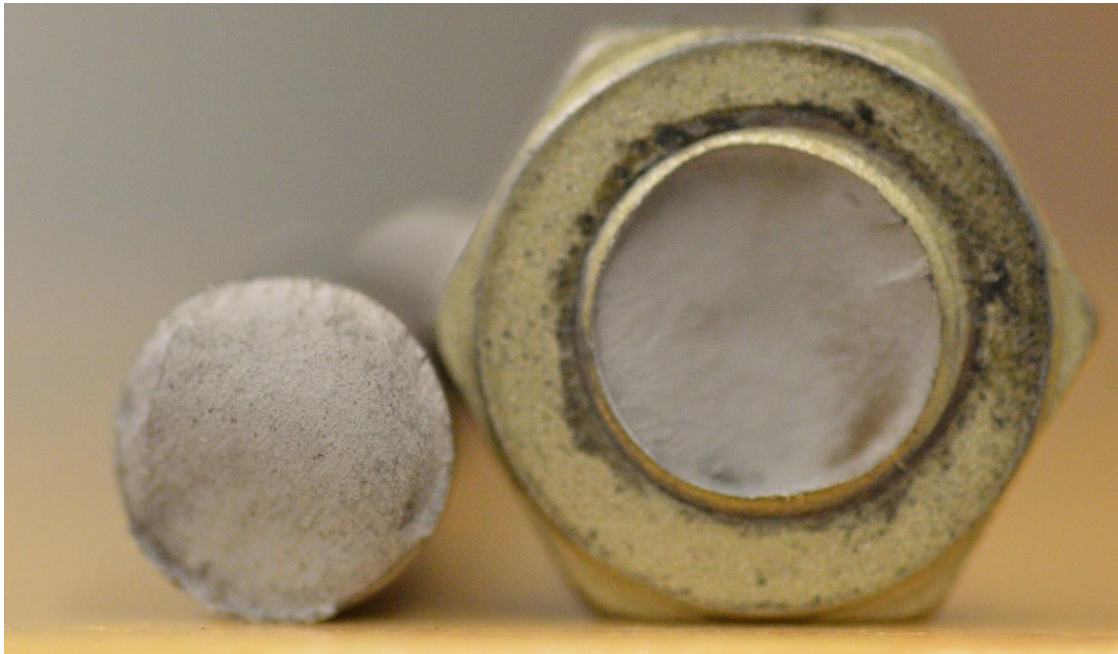
Figure 39: Fatigue failed fastener
