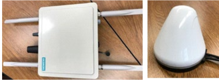
Figure 3.3. RSU (left) and OBU (right)
