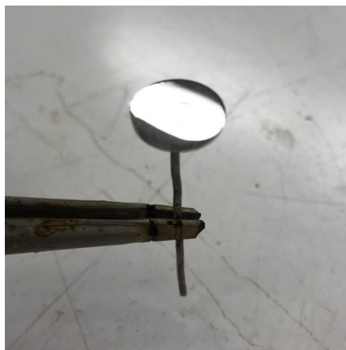
Figure A.1: Resulting electrode after polishing procedure.
