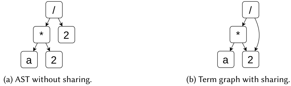
Figure 2.1: Different representations of the program (a * 2)/2 have different characteristics. The syntax tree is simpler (a), but the term graph is smaller since it captures sharing (b).
