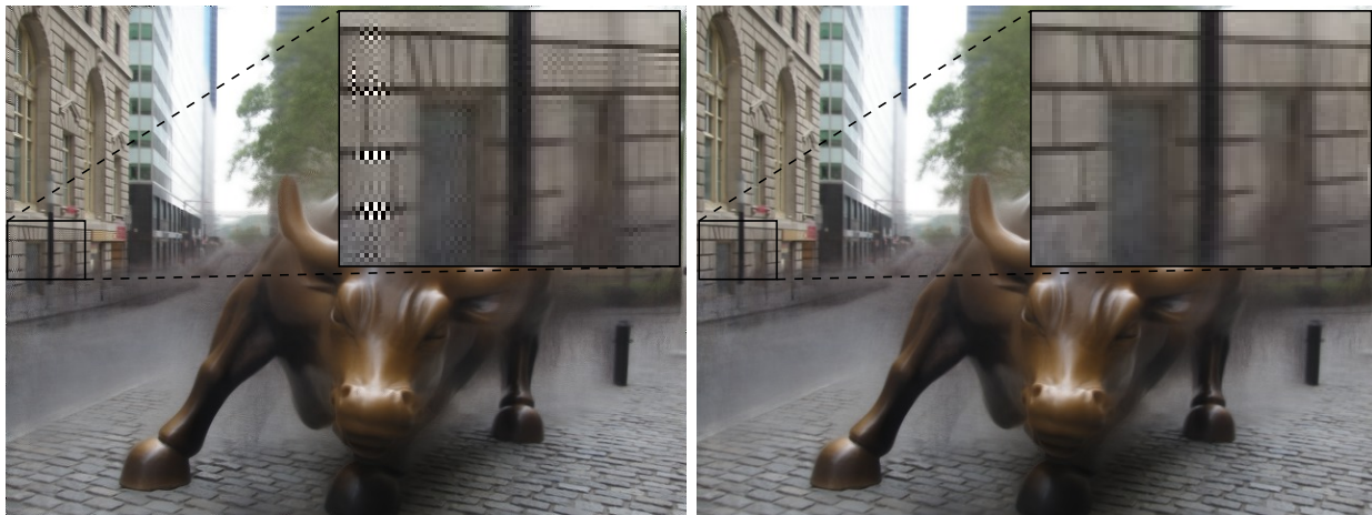
Figure 3.8: Comparison of different values of the 3D track sampling threshold \epsilon for the Wall Street Bull scene. Left: Artifacts are visible when \epsilon = 1 pixel, with alternating black and white pixels, as the reconstruction problem is badly conditioned. Right: Using \epsilon = 0.4 pixel, the artifacts are not present.
