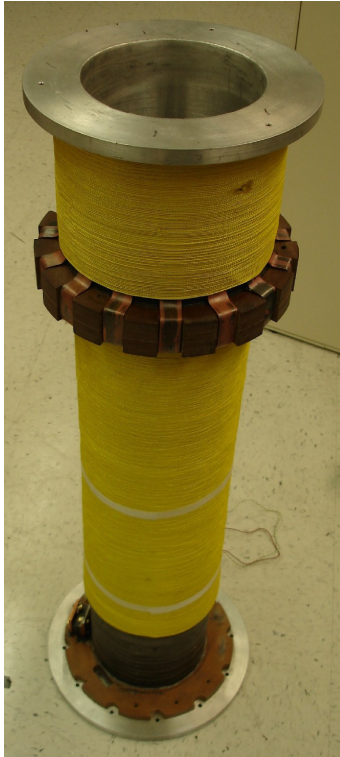
Figure 4.17: The bucking coil is a compound coil with a long, main solenoid to produce a zero-field volume and a counter-wound coil to eliminate any mutual inductance between the bucking coil and the main magnet. The epoxy potted, copper stabilized, niobium-titanium coils have a total inductance of around 4 Henries. It is welded inside the insert's LHe reservoir.
