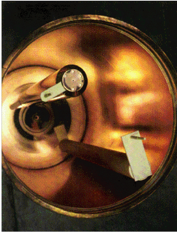
Figure 4.6: Left: a picture of the inside of an earlier ADMX cavity with tuning rods installed. Right: a sketch illustrating the tuning rods moving within the cavity. By rotating the alumina shafts of the tuning rods, the tuning rods are swung towards or away from the center of the cavity. With both rods near the center, the TM_{010} mode has a frequency of roughly 900 MHz. With both rods positioned closest to the cavity walls, the TM_{010} mode has a frequency of roughly 500 MHz.
