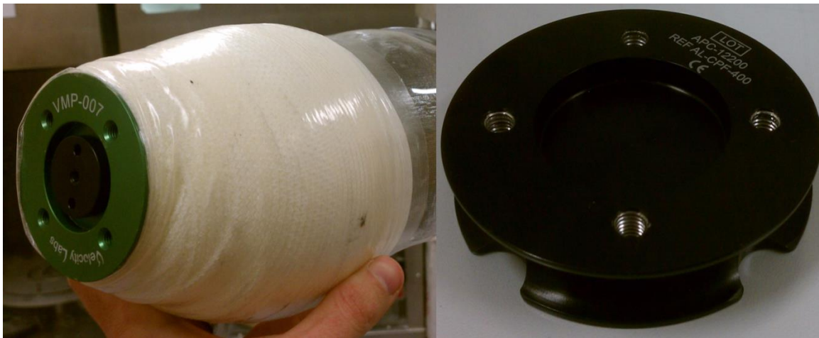
Figure 3: Attachment Plates for Lower Limb Prosthetics
