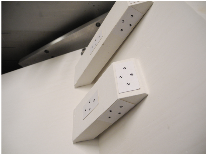
(b) Sliding blocks with varying aspect ratio that undergo sliding in back supported configuration (represents test 11).
