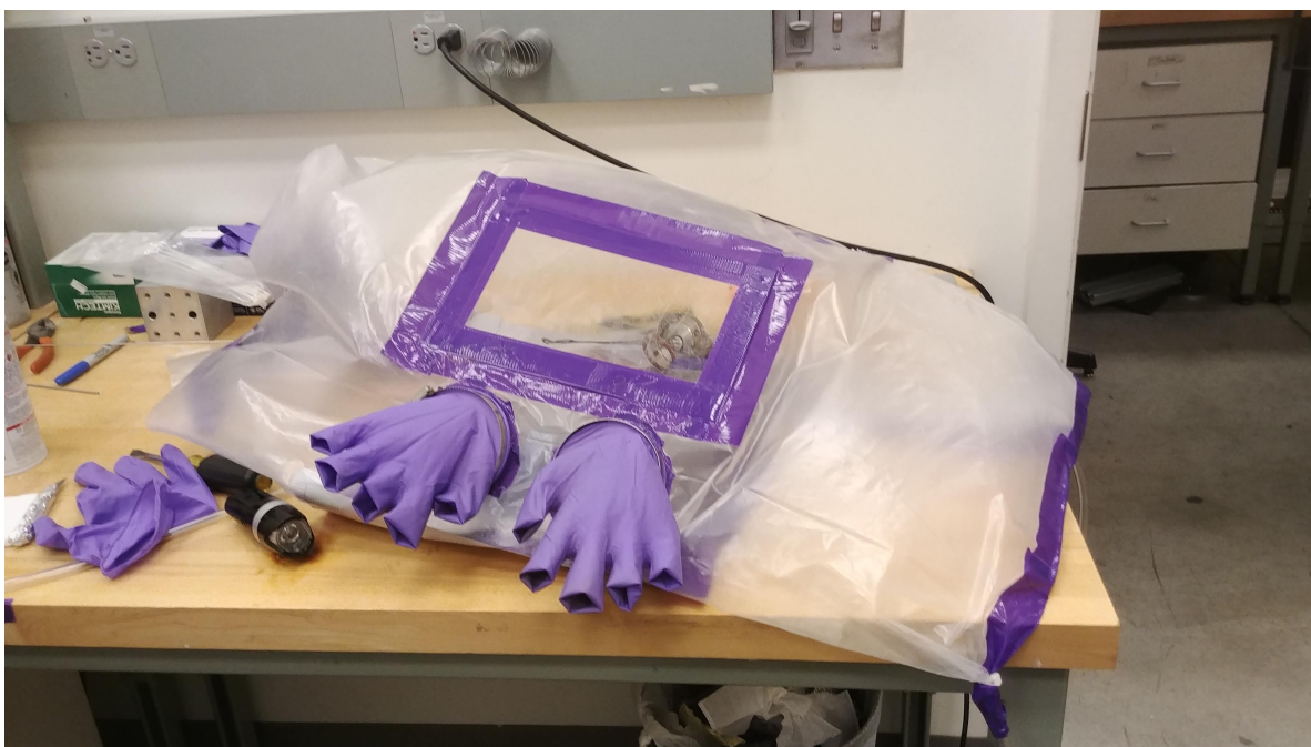
Figure 5.2: A glovebag was constructed to allow barium loading in an inert neutral gas. Gloved hands inserted into the attached XL gloves allowed for dexterous manipulation of the barium sample and oven. Tubing attached to the right corners of the bag allowed it to be filled from a gas cannister and pumped out with a roughing pump. A strip of tape on the backside of the bag (not visible) was used to seal a slit used for inserting and removing components.
