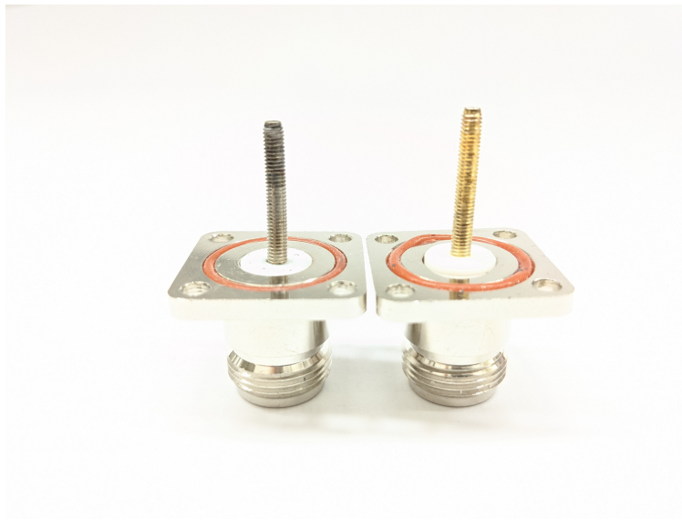
Figure 3.9: Image showing the zinc vaporization present in the threaded N type connectors after exposure to the thruster environment. The N type connector on the left was fired in vacuum, while the connector on the right was not.
