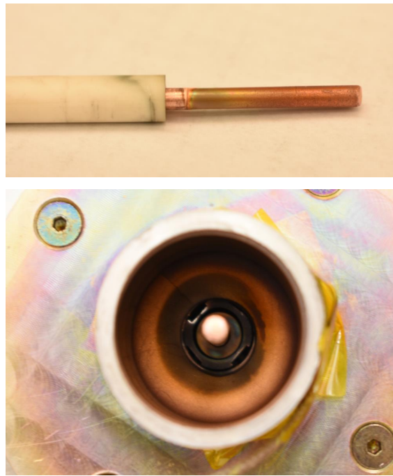
Figure 3.18: The patinated copper antenna, showing the demarcation between the protected and exposed sections of the antenna (top) and copper deposition on the thruster components (bottom).
