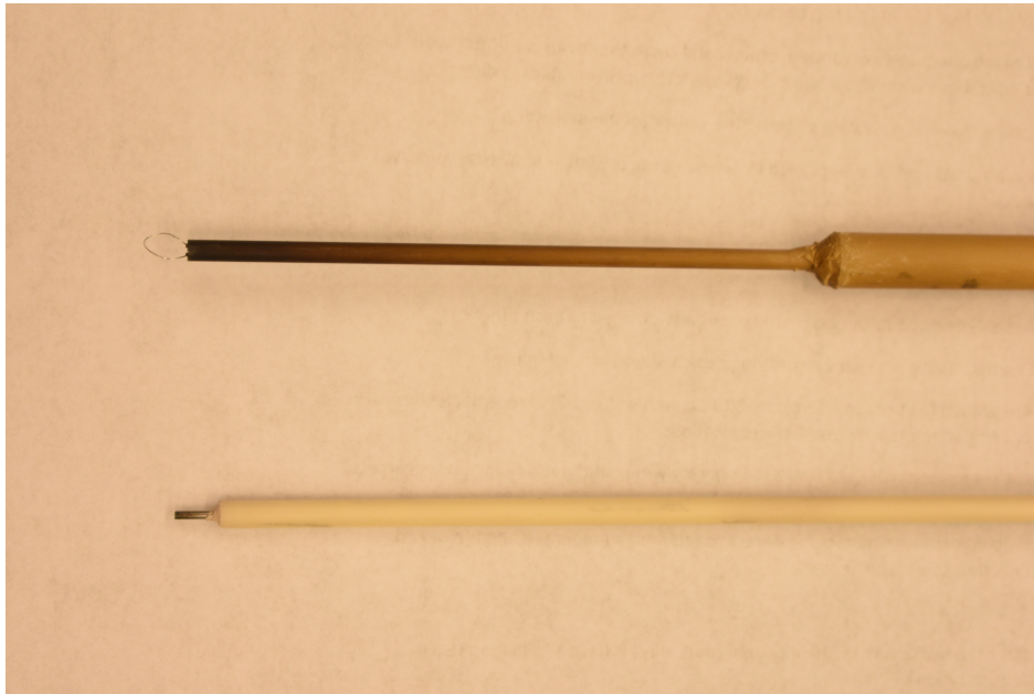
Figure 3.23: Image of the emissive (top) and Langmuir (bottom) probes used in testing.
