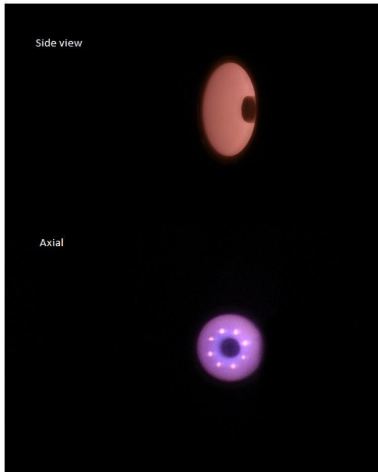
Figure 3.7: 45° angle side (top) and end-on (bottom) view of plasma forming in the plenum region of the thruster.
