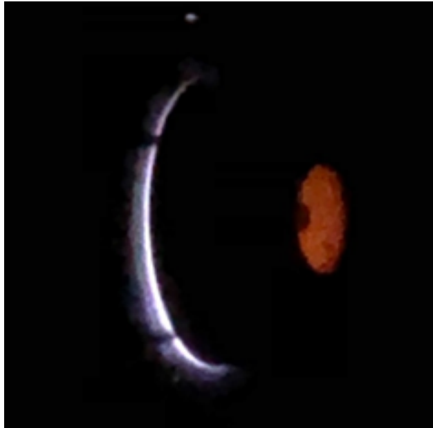
Figure 3.6: Image of plasma forming in the plenum region of the thruster.
