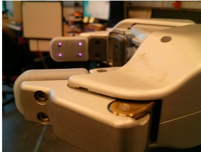
Figure 3.14: The IR beam optical pretouch sensor on the PR2 robot.
